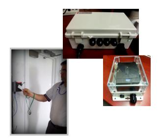
Advatek Scanpad controller is a basic solution to allow employee in and out times to be captured for timekeeping or door access control applications. There is no display or keypad to protect, so the controller can be installed in just about any environment. A Scanpad controller can monitor up to four badge readers, with each badge reader being configured as an IN or OUT scan station. This is an option when it is not necessary for the employee to input data or make onscreen selections.
