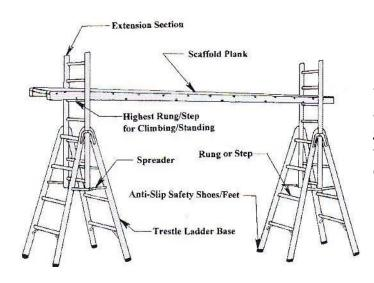
The maximum length of a ladder measured along its side rail <u>shall not be more than 5</u> metres for a trestle ladder or for each of the base and extension sections of an extension trestle ladder.
