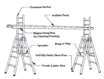
The maximum length of a ladder measured along its side rail <u>shall not be more than 5</u> metres for a trestle ladder or for each of the base and extension sections of an extension trestle ladder.
