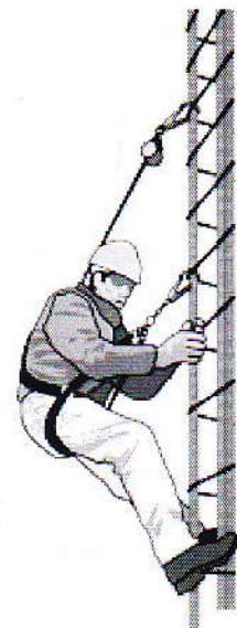
A positioning-device system with self-retracting lifeline
