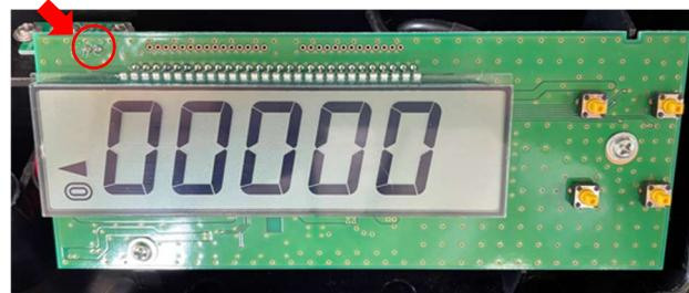
In test mode, the following types of the internal count are displayed. When the **[ $\leftarrow$  T  $\rightarrow$ ]** key is pressed, the internal count, power supply voltage, display check and others are cyclically shown on the panel in the following order.
