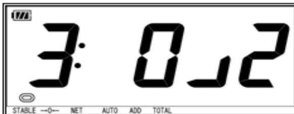
Adjustment made using 3 points – zero point, 1/2 weighing capacity and full weighing capacity
