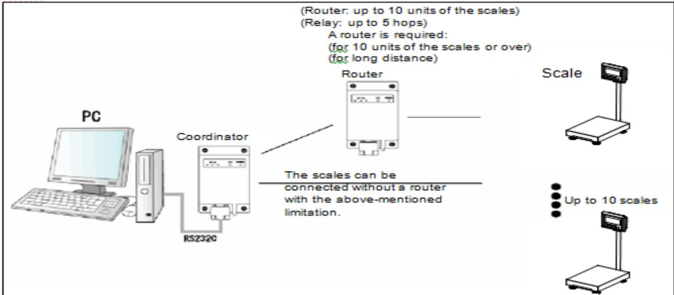
A transmission/reception device called a coordinator is connected to a PC for communication. Each scale has a built-in a ZBee board (called an end device) for the communication with the coordinator. Unlike the Bluetooth communication, no pairing is required between a coordinator and a scale. A coordinator is capable of communicating with any scale that are detected by it.
