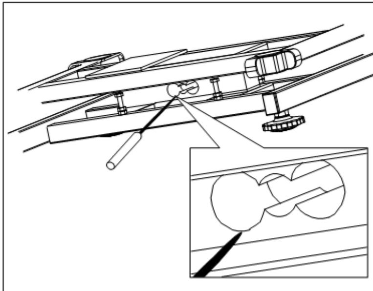
Figure 3-4 View of Eccentric Error Adjustment
