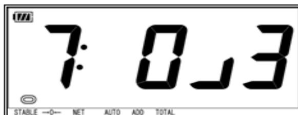
Adjustment made using 4 points – zero point, 1/3 weighing capacity, 2/3 weighing capacity and full weighing capacity
