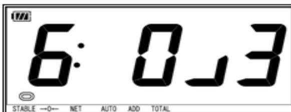
Adjustment made using 4 points – zero point, 500 increments, 2/3 weighing capacity and full weighing capacity
