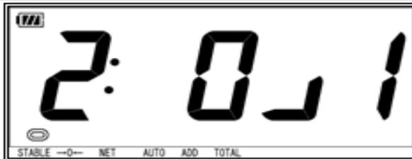
Adjustment made using 2 points – zero point and full weighing capacity
