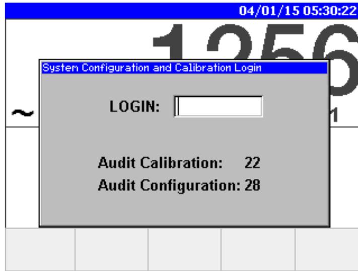
The login screen displays the APX software version as well as the Calibration and Configuration Audit Trail counters for metrological sealing of the device.
