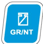
**GR/NT:** **GR/NT** - Toggles between GROSS and NET weighing modes if a tare value is stored.
