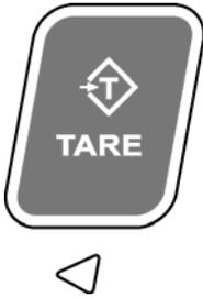
Press the key: **TARE** - Acquires tare value from weight on the scale (Container, Box, etc.)
