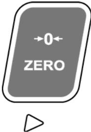
Press the key: **ZERO** – Sets the weight display to zero.
