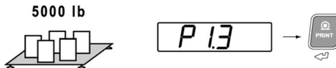
6. “SPAn” is briefly displayed. Enter the test weight amount using the **ARROW** keys to select and alter digits. Press the **ENTER** key to confirm the test weight value.
