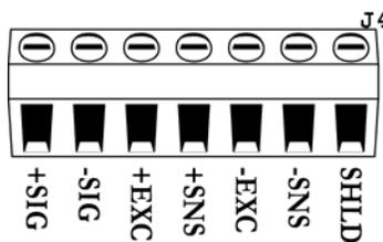
Fig. 4: Load Cell Terminal
