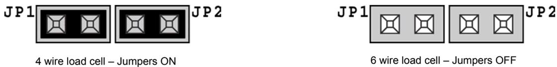
Fig. 5: Load Cell Jumpers
