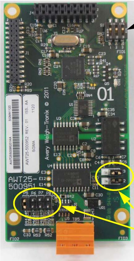
The analog output card uses a 16 bit A/D with resolution capabilities of 65,536 divisions.
