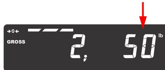
Above is a typical example of using a scale token. Upon creating the token, **t1** for Gross weight, the indicator automatically appends an additional number in the next character location. The value of the number in this next location identifies what function of the token is being used.
