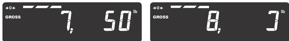
Characters 5 to 8 will remove the decimal point from the weight transmitted using an attribute parameter. You may need to refer to the *Network tokens* on [page 125](#) for more detail on necessary character values.
