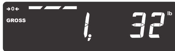
3. Press **SELECT** and the display will show the center bar segments flashing as well as the right digit. This shows you are in the editing mode.
