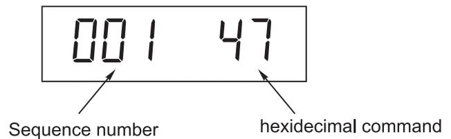
These numbers represent the default print format in numbered sequence of hexadecimal commands. Each hexadecimal command represents one printing character or print command. These numbers allow you to customize the print output of the indicator.
