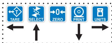
Press the ZERO (ESC) key to abort calibration.
