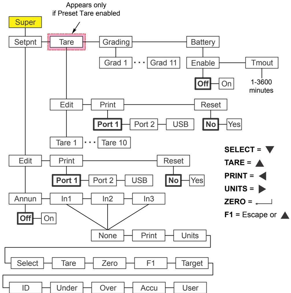
Figure 7.5 Supervisor menu for the Grad375 application
