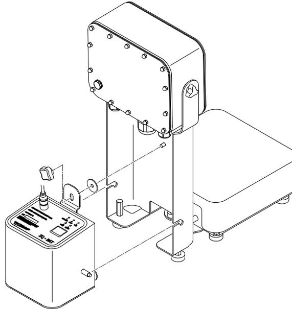
**Figure 2.7 ZQ-BAT installation**
