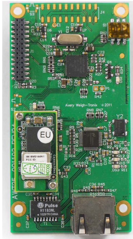
Figure 8.5 802.11g wireless communication option module
