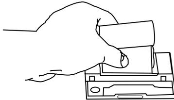
6. While holding the paper in place, press the rocker switch to the Paper Feed position. The printer will activate, and a rubber roller will pull the paper into the printer compartment. Hold the switch in the Paper Feed position until the paper emerges from the top of the printer mechanism.
