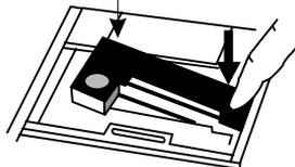
5. Install cartridge. Be sure the ink cartridge is inserted firmly to prevent weak or irregular printing. The cartridge must be properly seated and aligned for best printing.
