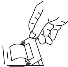
11. Press the front of the printer cover down to lock in place.
