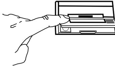
3. When the printer cover is tilted up, lift it completely off.
