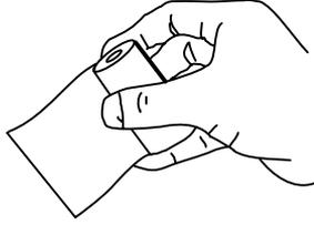
4. Cut a straight edge on the paper roll if it is jagged. This will facilitate the entry of the paper into the printer.
