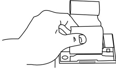
9. Slide the paper through the slot in the printer cover.
