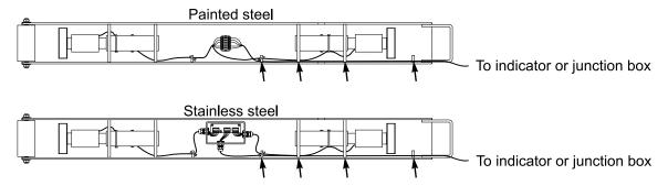
Connect the wires of the cable to the appropriate positions of the terminal block or junction box as determined by the connection chart below. +Sense must be connected to the same position as +Exc at the beam and/or extra junction box. Also, the -sense must be connected to the same position as -Exc. The cable may be secured in place with the supplied cable ties.
