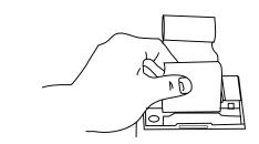
9. Slide the paper through the slot in the printer cover.
