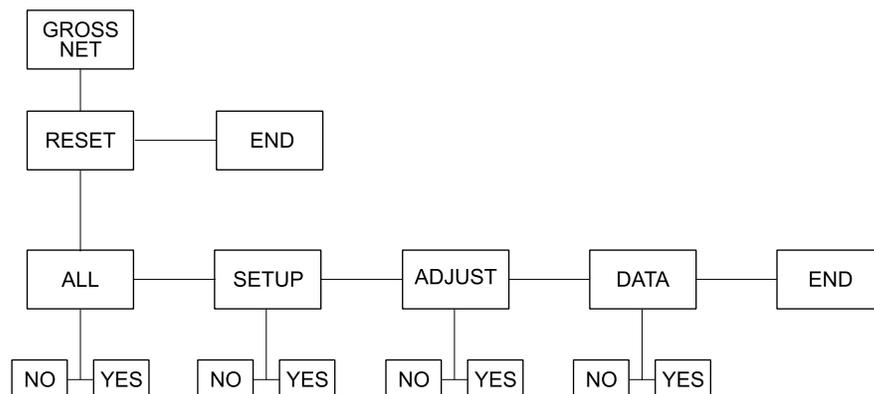
If *SETUP*, *ADJUST*, or *DATA* appears and it is flashing, the indicator is telling you that it is corrupted and must be reset to default values.
