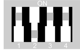
WI-150's ON/OFF keys to the appropriate circuitry, should always be in the ON position to allow optimal functioning of the indicator. S1-2 is not functional.
