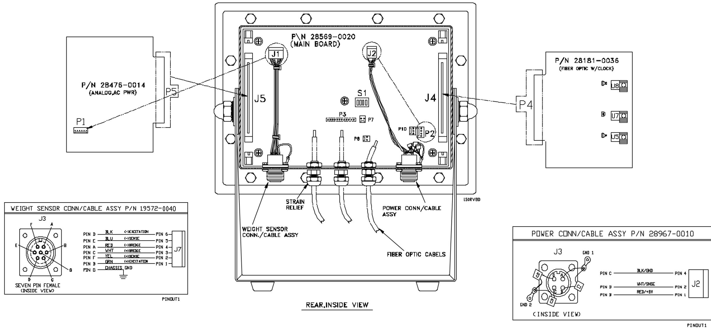
**WI-150 AC/DC INDICATOR (BATTERY POWERED)**
