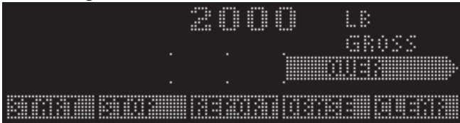
Checkweigher shown in overload condition below.
