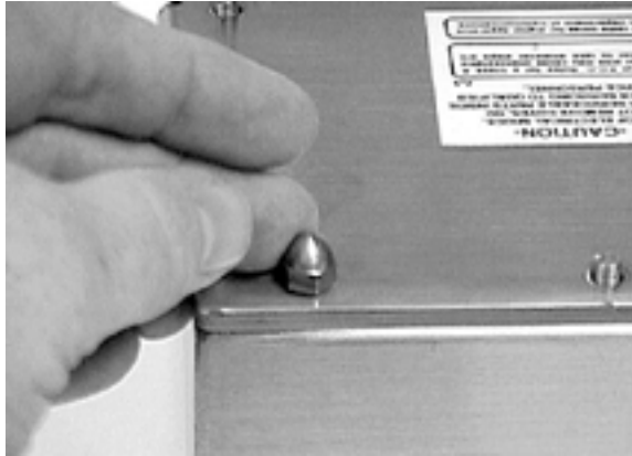
Figure 10 Removing acorn nuts
