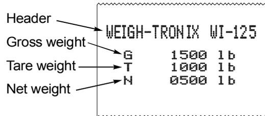
A rectangular box with a dashed border containing a printout. On the left, four labels have arrows pointing to specific characters in the printout: "Header" points to "WEIGH-TRONIX", "Gross weight" points to "G", "Tare weight" points to "T", and "Net weight" points to "N". The printout text is as follows:
