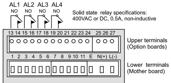
*Both analogue output option and trips option is available on one instrument. Refer to the appropriate sections of the manual for wiring information.*
