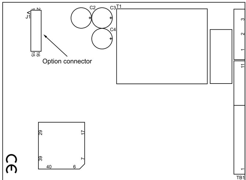
The analog output option is a separate circuit board that is fitted in the upper slot of the instrument housing. The upper board and terminals are clearly numbered 13-28 to differentiate them from the lower terminals.
