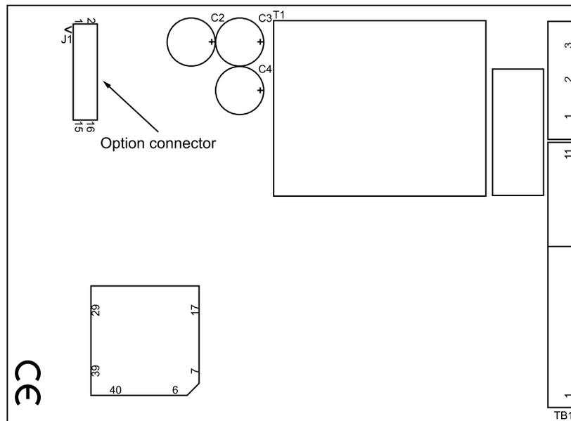
The trip relay option is a separate circuit board that is fitted in the upper slot of the instrument housing. The upper board and terminals are clearly numbered 13-28 to differentiate them from the lower terminals.
