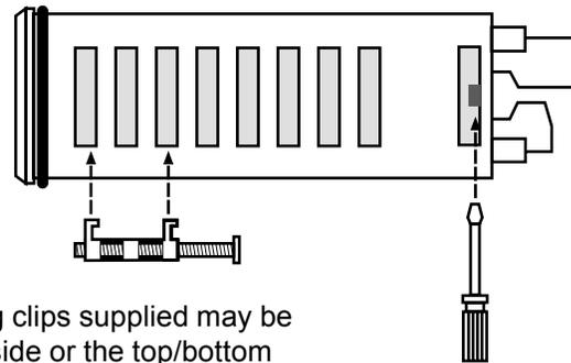
The fastening clips supplied may be fitted on the side or the top/bottom of the instrument. Ensure that the clip and screw is mounted as shown here. **Do not overtighten the screws.**
