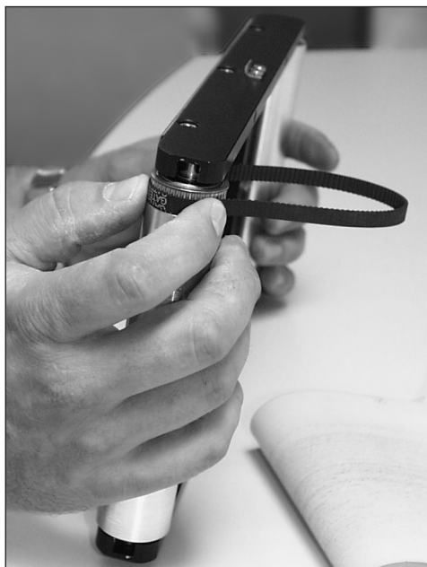
Fig. 31: Replacing the toothed belt
