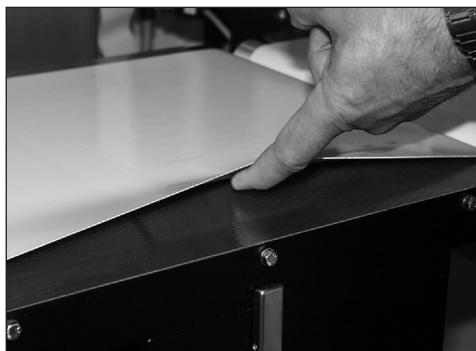
Fig. 8: Sufficient belt tension (one-finger rule)
