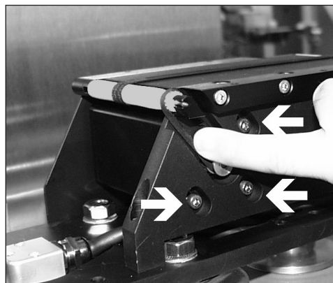
Fig. 27: Motor fixation of the weighing conveyor
