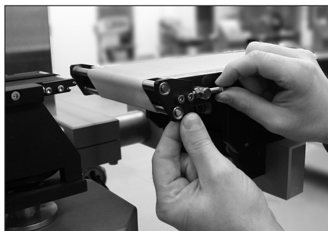
Fig. 10: Example: Belt tensioning screw at the infeed conveyor
