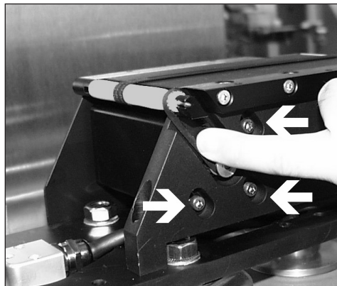
Fig. 18: Hexagon screws of the motor fixation
