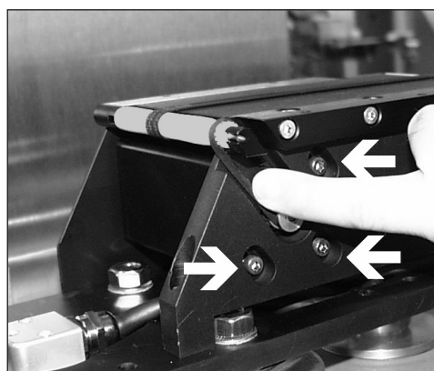
Fig. 28: Hexagon screws of the motor fixation
