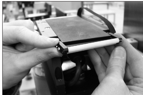
Fig. 20: Removing the idle roller holder
