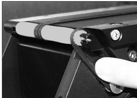
Fig. 26: Checking the toothed belt tension
