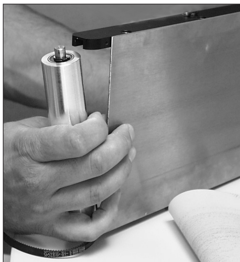
Fig. 24: Replacing a roller
