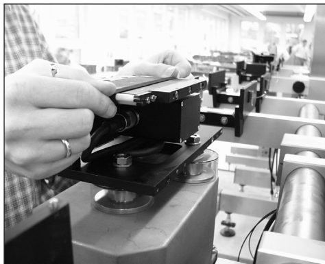
Fig. 7: Replacing the transport belt
