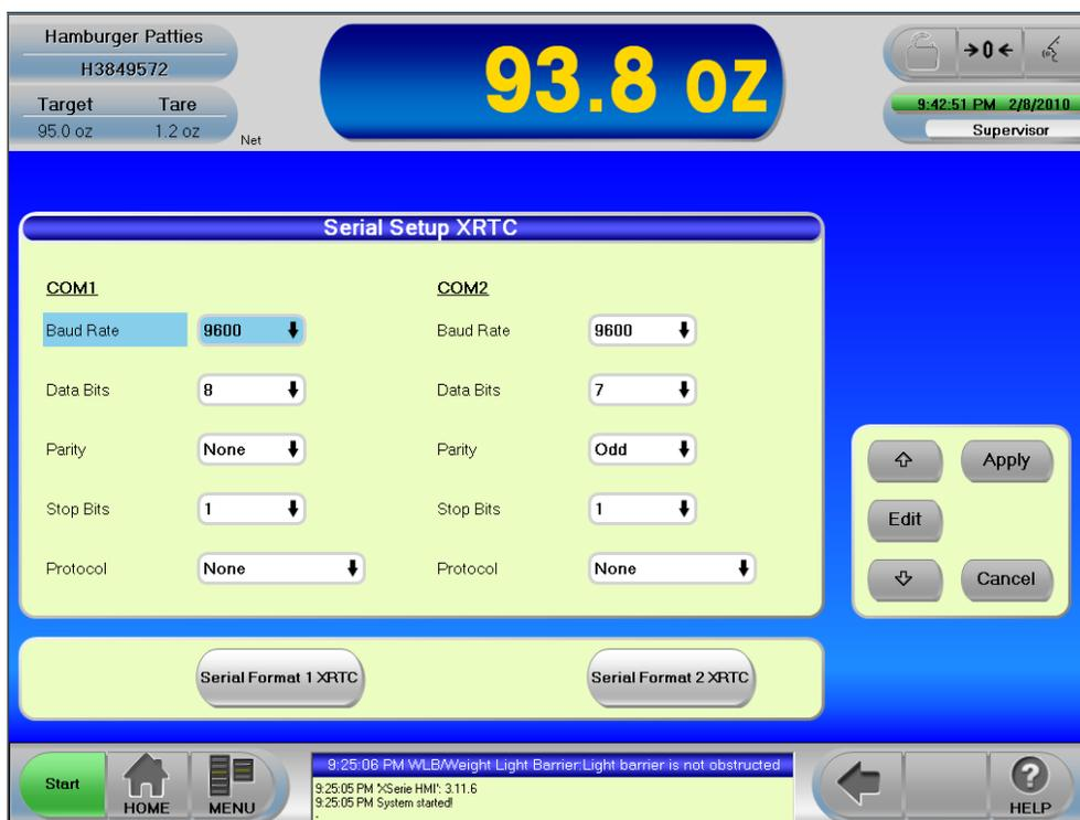
Figure 11.3: Serial Setup XRTC
