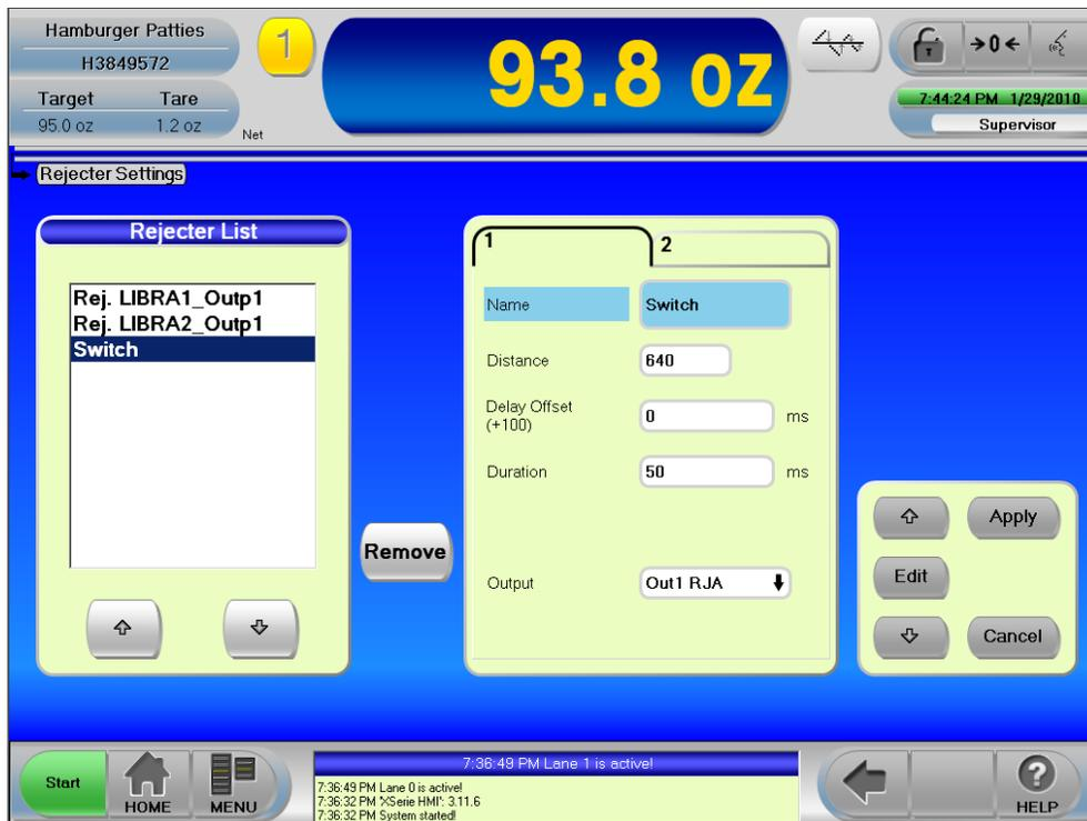
**Figure 5.3: Rejecter Removal Screen - Tab 1**
