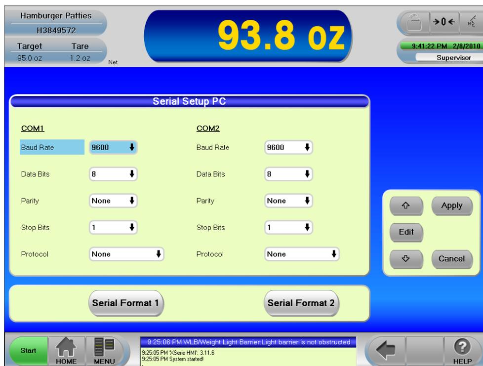
Figure 11.2: Serial Setup PC Screen
