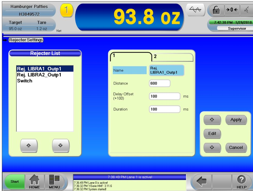
Figure 5.2: Rejecter Setup Screen - Tab 1
