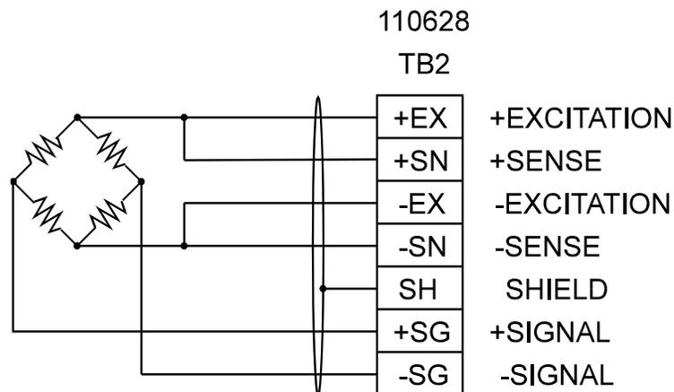
FIGURE 1-2 LOAD CELL TERMINATION
