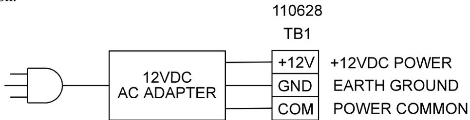
FIGURE 1-1 POWER SUPPLY CONNECTION
