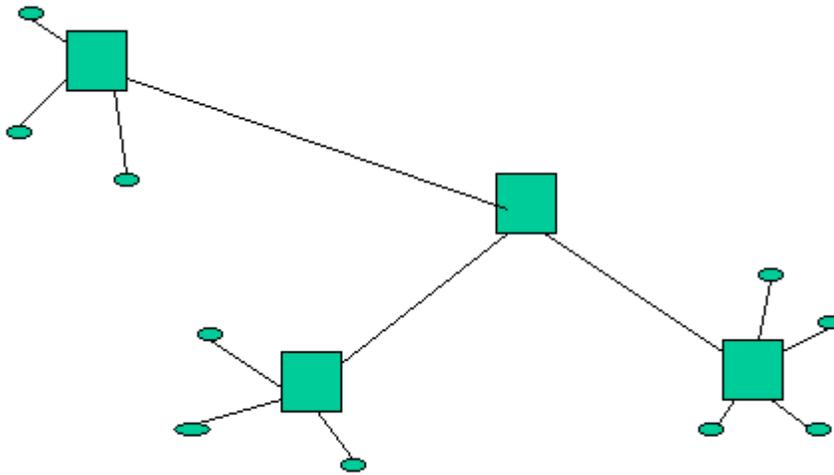
USB uses a “Star” topology, which means that there is only one device connected at each end of a cable, and multiple devices require a hub to re-distribute the signal.
