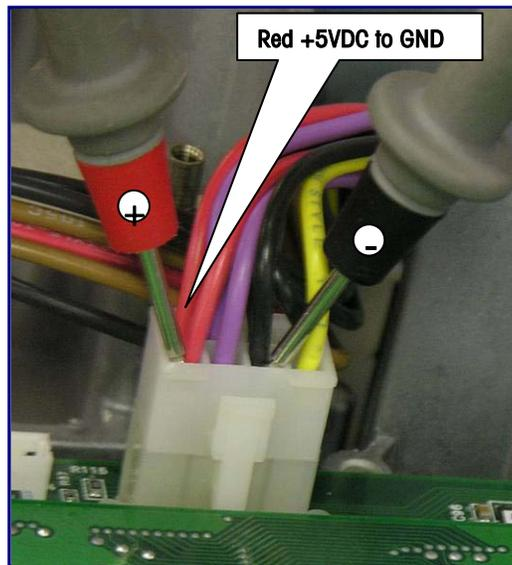
Figure 4-3: (+5VDC Range: +4.5 VDC to +5.5 VDC)
