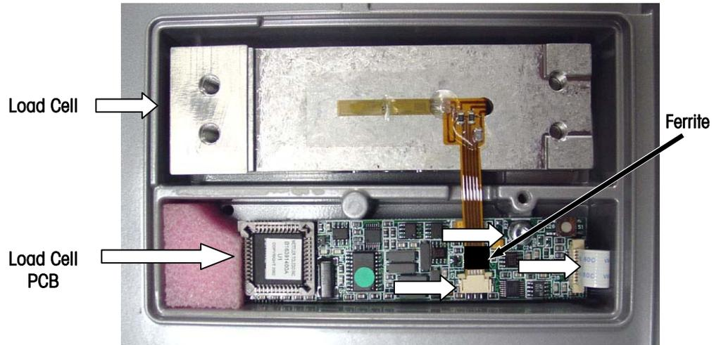
**Figure 4-15: Standard - Load Cell and Load Cell PCB**
