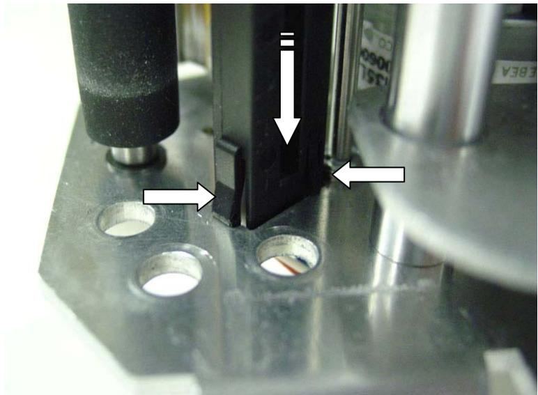
**Figure 4-32: Gap Sensor Spring Clips**
