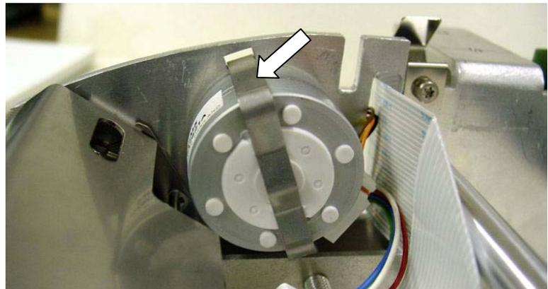
Figure 4-26: Label Stepper Motor and Mounting Clip (Label Side)
