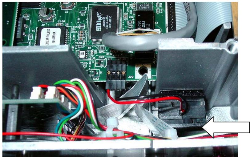
Figure 4-6: Main PCB Battery
