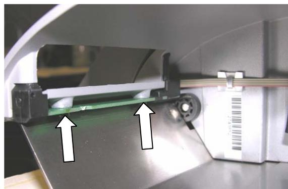
Figure 4-29: Take Label Sensor (inside view)
