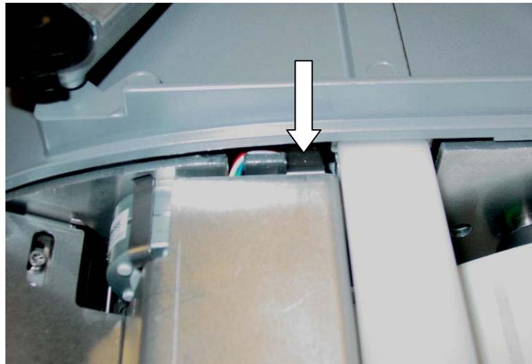
Figure 4-20: Printer Stop Tab
