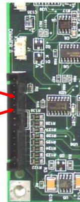
Figure 4-8: LCD Contrast/Voltage Test Points on Main PCB
