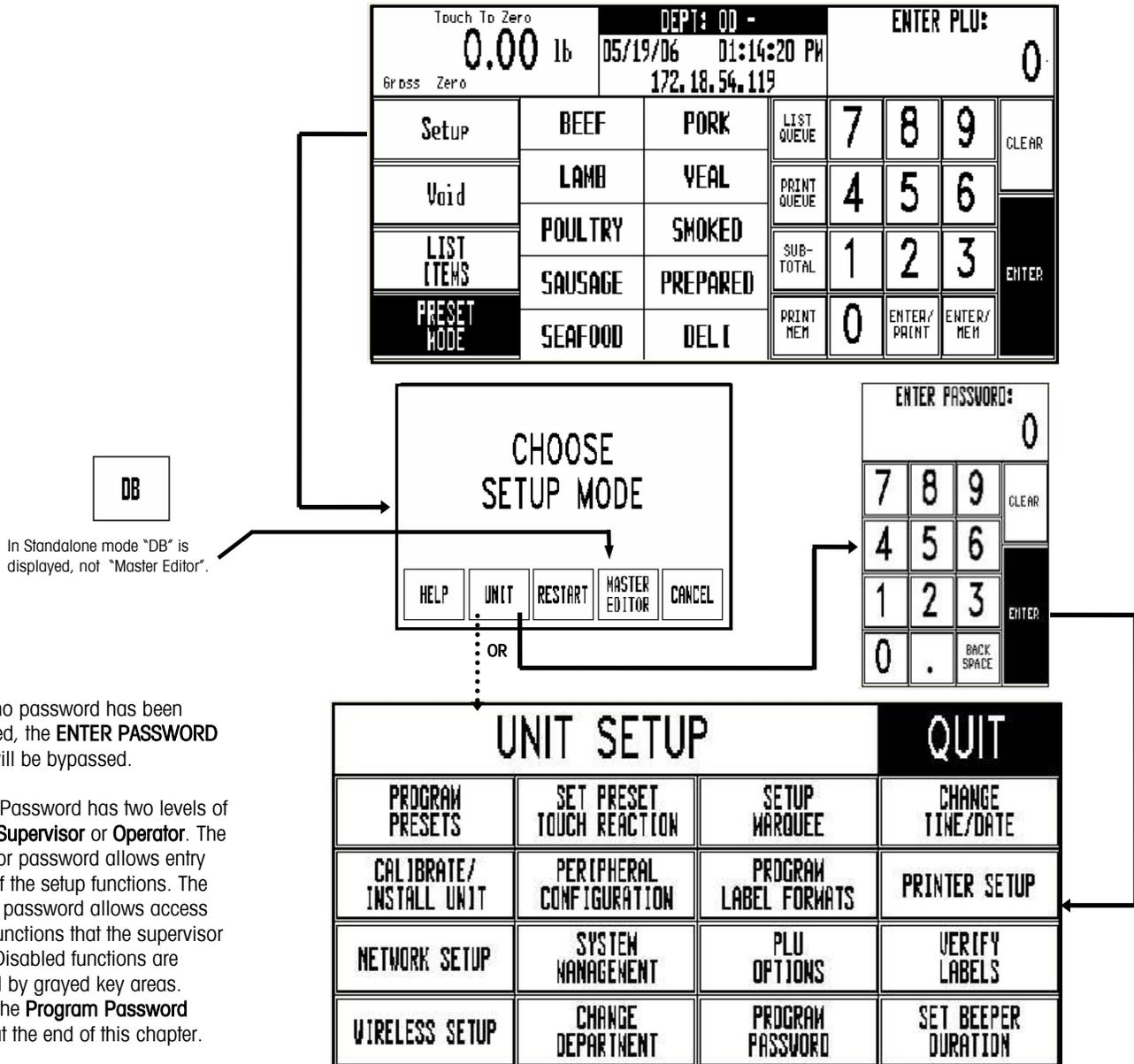
Figure 3-1: Unit Setup
