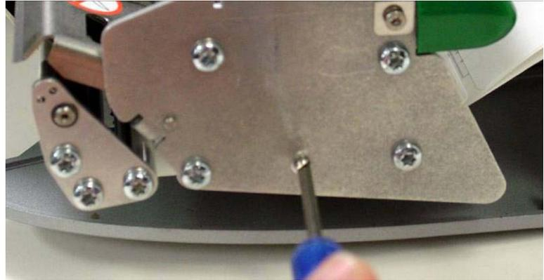
Figure 4-34: Guide Adjustment
