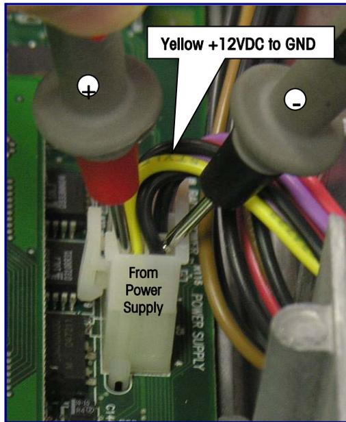
Figure 4-2: (+12VDC Range: 11.5 VDC to 14.5 VDC)
