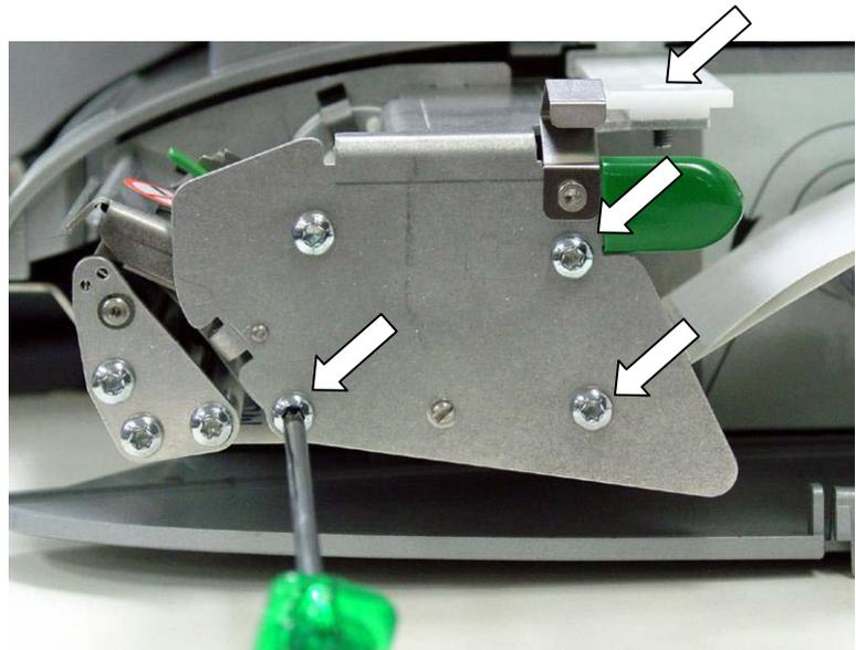
Figure 4-25: Printer Side Plate Removal
