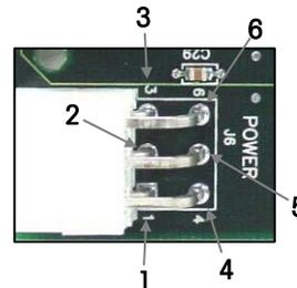
Figure 4-24: Testing +24VDC and +5VDC from Power Supply
