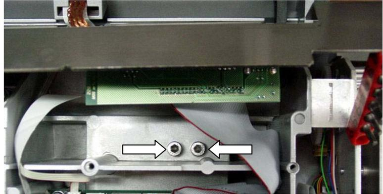
**Figure 4-17: Lower Load Cell Mounting Screws**
