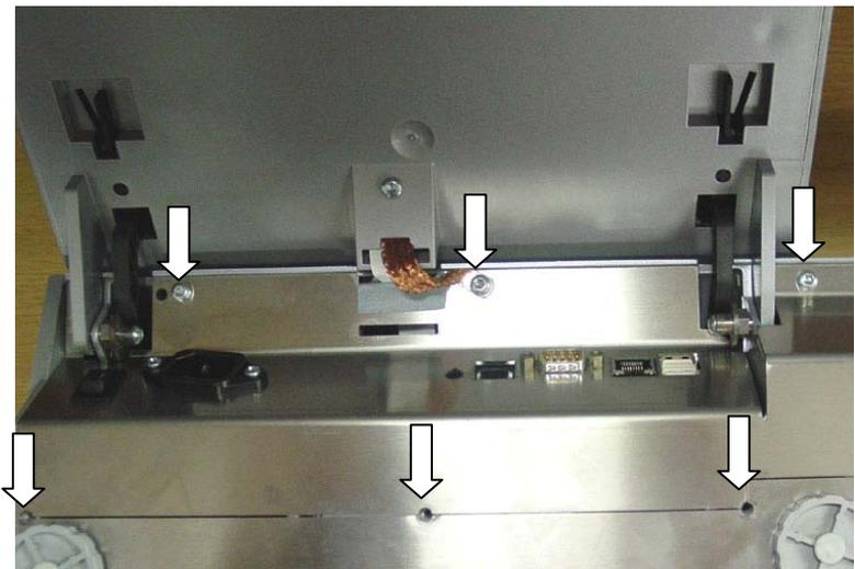
**Figure 4-16: Bottom Cover Removal**
