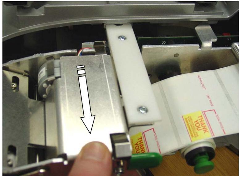
**Figure 4-21: Printer Slide Rail**
