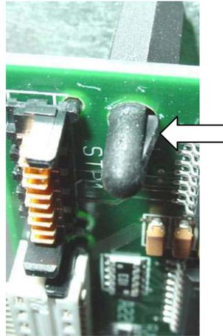
Figure 4-23: Printer PCB Standoff and Locking Clips
