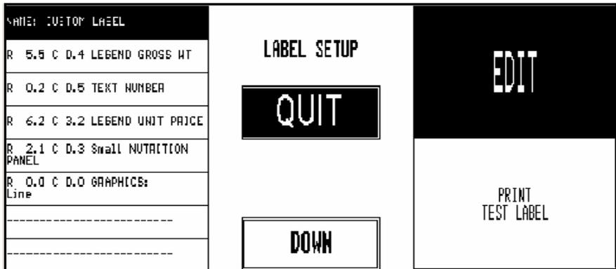
Figure 3-14: Field Setup with Label Entities
