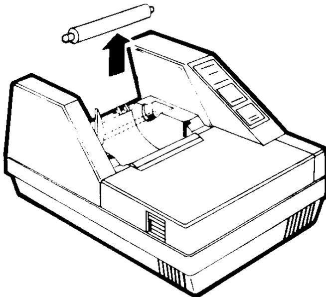
Figure 3.5 - 2 Removing Paper Axle
