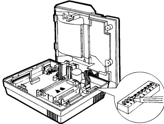
Figure 4.1.2 Set Programming Switches
