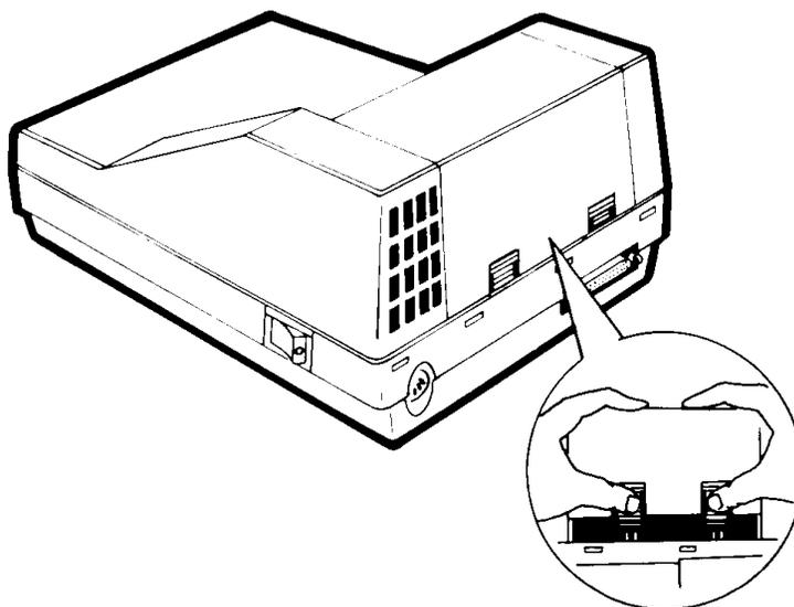
Figure 3.5 - 1 Removing Paper Tray Cover
