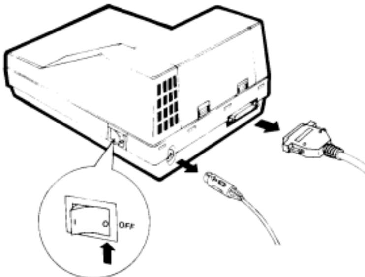
Figure 4.1.1 - 2 Turn Power Off, Disconnect All Cables
