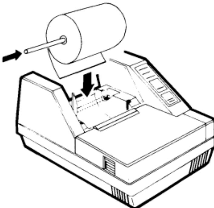
Figure 3.5 - 3 Installing Paper Roll
