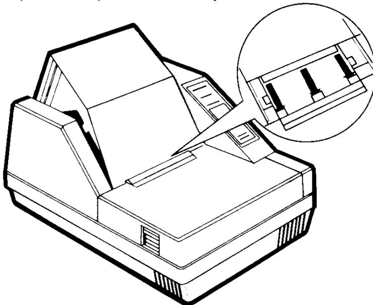
Figure 3.6 - 2 Replacing Rear Paper Cover
