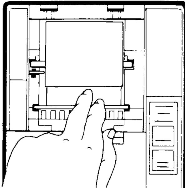
Figure 3.5 - 4 Threading Paper
