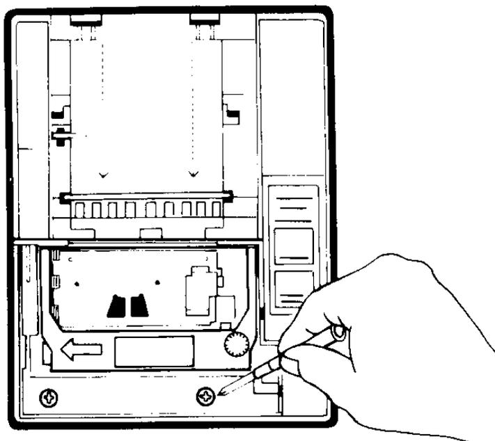
Figure 4.1.1 - 4 Remove Mounting Screws
