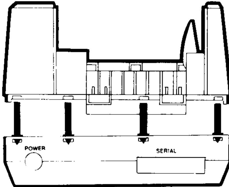
Figure 4.1.3 - 1 Close Printer Enclosure
