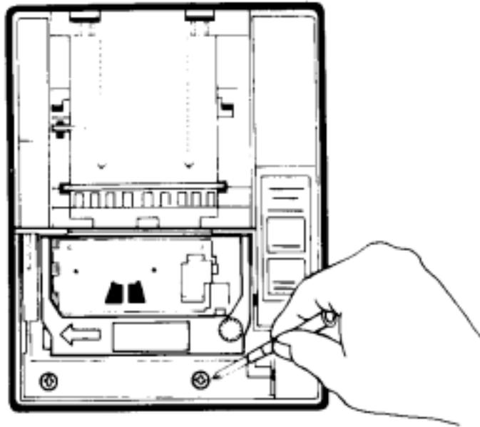
Figure 4.1.3 - 2 Reinstall Mounting Screws
