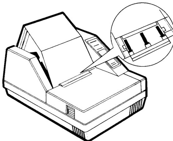
Figure 4.1.3 - 5 Reinstall The Paper Tray Cover
