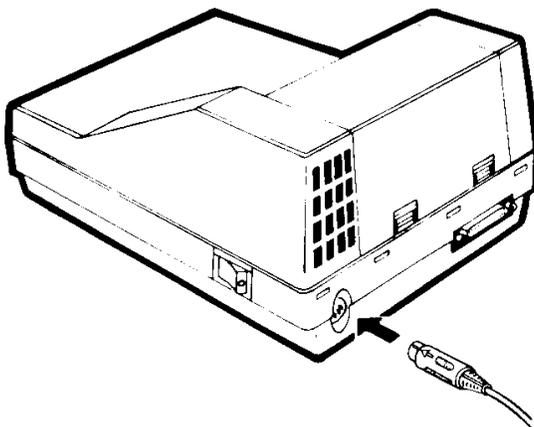
Figure 3.3 Connect Power Cable
