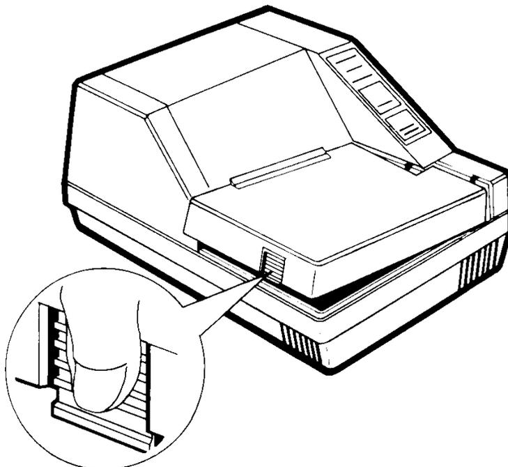
Figure 3.2 - 1 Removing Front Cover
