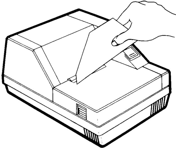
Figure 3.7 Tearing Off the Printed Portion
