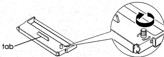
Insert the cartridge as shown below, making sure it snaps in place. The ribbon must be between the printhead and platen. Turn the knob to take up any slack. Close the printer cover.
