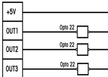
The output voltage at Logic 0 is .4VDC maximum with sink current of 8mADC or less. The output voltage at Logic 1 is 4.0VDC minimum with source current of 8mADC or less. The discrete outputs are capable of driving solid state relays and are typically used with these devices to switch various DC voltage levels, 110 VAC or 220 VAC. The solid state relay is activated (on) when the SpeedWeigh/SpeedWeigh Plus scale output is at Logic 0 and deactivated (off) when the output is at Logic 1.
