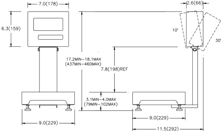
The SW06/SW06K base measures 79 mm (3.1 in.) high x 229 mm (9.0 in) wide x 229 mm (9.0 in) deep. The overall height is 437 mm (17.2 in) and overall depth is 292 mm (11.5 in) with the standard column.
