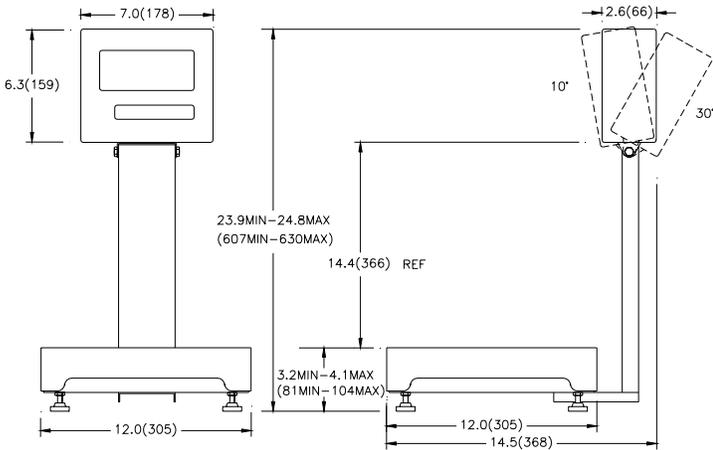
These bases measure 81 mm (3.2 in.) high x 305 mm (12.0 in) wide x 305 mm (12.0 in) deep. Overall height is 607 mm (23.9 in.) and overall depth is 368 mm (14.5 in.) with the standard column.
