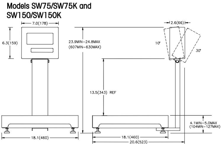
These bases measure 104 mm (4.0 in.) high x 457 mm (18.0 in) wide x 457 mm (18.0 in) deep. Overall height is 600 mm (23.6 in).
