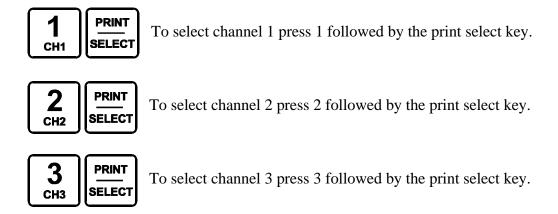
Note: that by default only channel 1 is enabled. To enable channels 2 and 3 you must enter calibration mode and use parameter 98 to enable them. Trying to select a scale channel that is not enabled will display error message 40.
