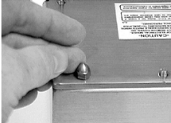
Figure 10 Removing acorn nuts
