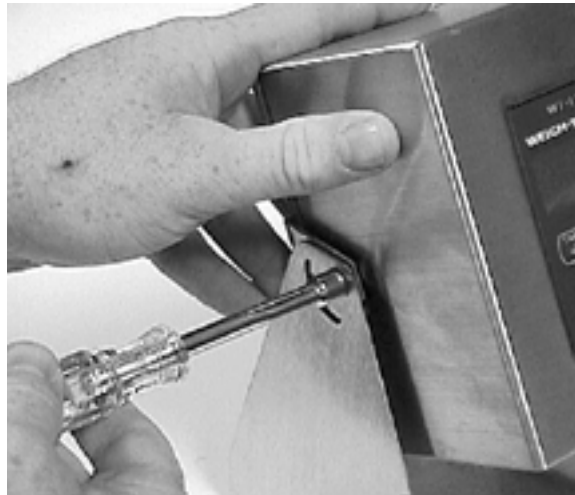
Figure 9 Removing stand screws
