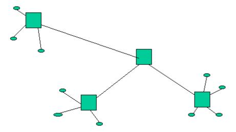
USB uses a "Star" topology, which means that there is only one device connected at each end of a cable, and multiple devices require a hub to re-distribute the signal.
