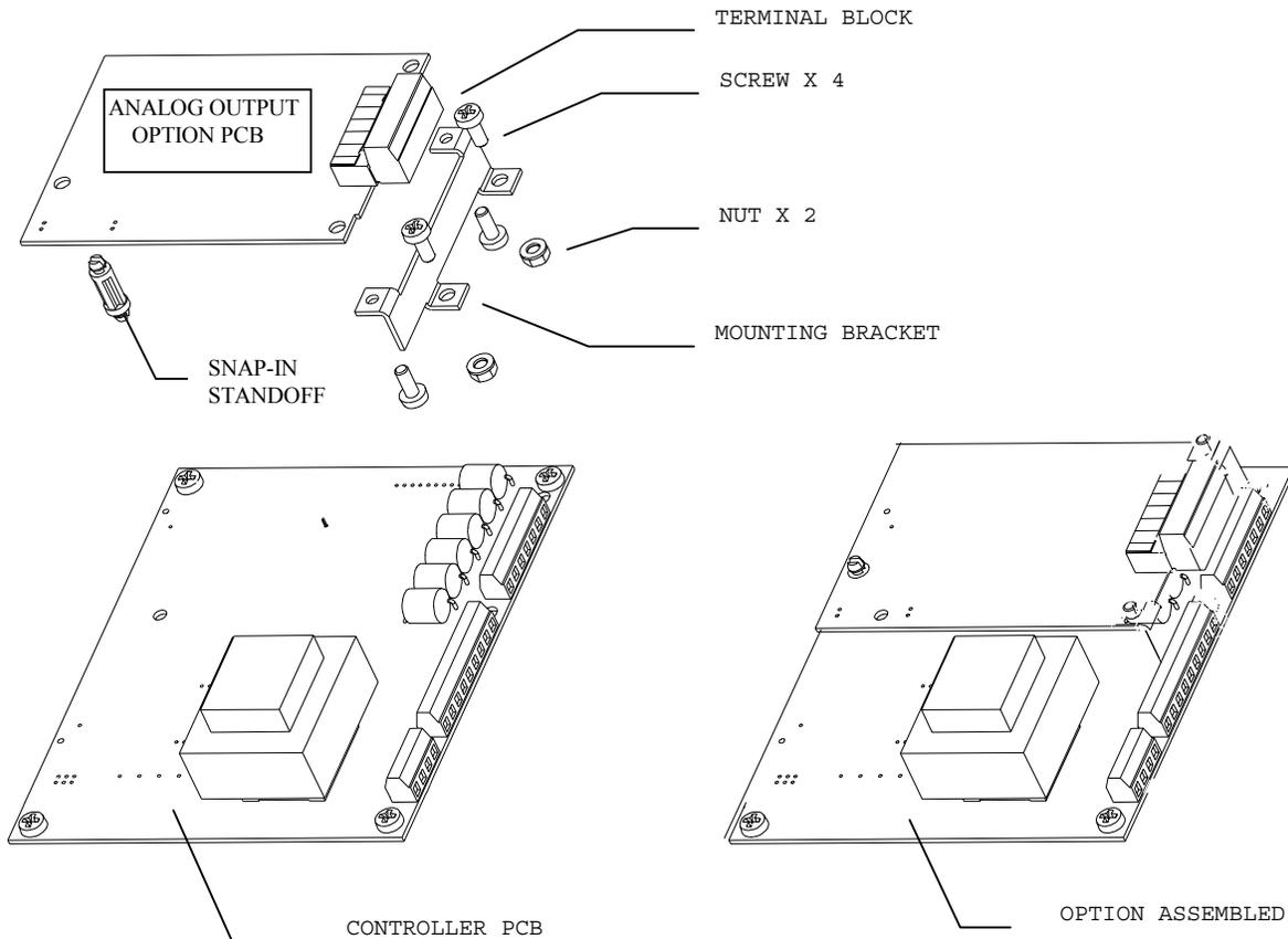
4. The mounting bracket is attached to the Analog Output Option PCB with two screws.
