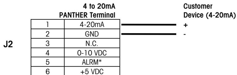
Note: The output from the analog module is fixed at absolute displayed weight.
