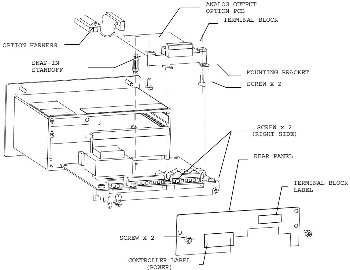
10. Plug the option harness into the Analog Output Option PCB at J1.
