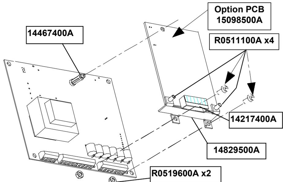
Figure 6-2 Allen-Bradley PCB Installation in Panel Mount Enclosure
