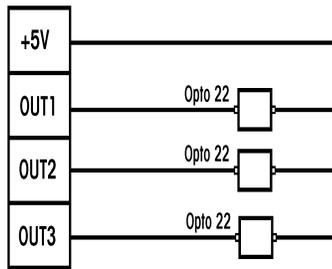
The discrete outputs may be used in conjunction with either the setpoint mode or over/under mode.
