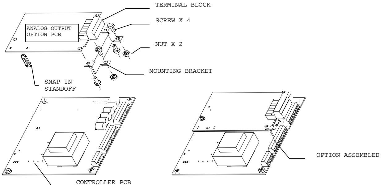
4. Remove the two screws on the right securing the Controller PCB to the Controller PCB mounting bracket. (Leave the one on the left alone.)
