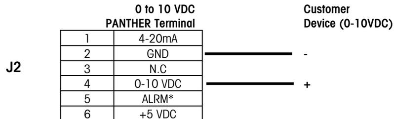
The ALRM Output (Alarm) is an open collector output. If the PANTHER terminal weight display goes to an over capacity or under zero display, or Setup is entered, the connection closes and the ALRM Output will be capable of sinking up to 30 mA DC to ground. The voltage source can be the +5V supplied with the Analog Output PCB or a maximum of +30 VDC external source.
