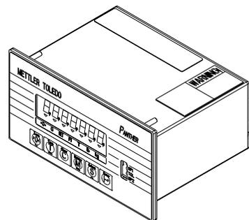
The panel-mount PANTHER terminal model measures: 3.62 in. (9.2 cm) high × 6.75 in. (17.1 cm) wide at the front and 5.20 in. (13.2 cm) deep. Refer to the cutout diagram when installing the panel-mount PANTHER terminal. Note: The optional high-level optos add 1.25 in. (3.17 cm) to the depth.
