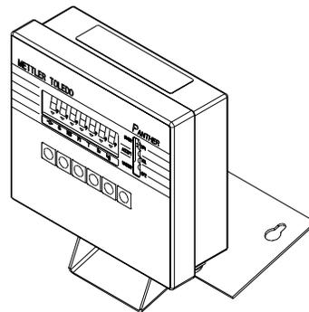
The PANTHER harsh environment terminal measures: 15.9 cm (6.25 in.) high × 17.8 cm (7.00 in.) wide at the front of the terminal and is 6.6 cm (2.59 in.) deep. The location of the keyholes for wall mounting screws is shown in the illustrations on the next page.
