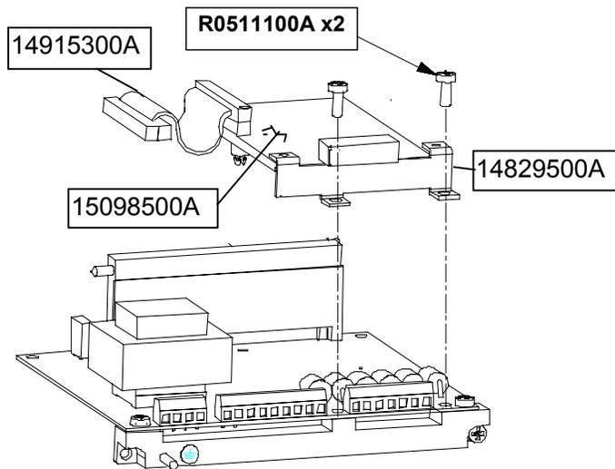
Figure 6-3 Allen-Bradley PCB Installation in Panel Mount Enclosure
