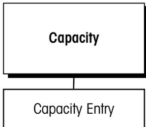
The Capacity sub-block lets you enter the maximum scale capacity. The capacity is given in the calibration units. The weight display will indicate **OVER RANGE** at 5 increments above this weight.
