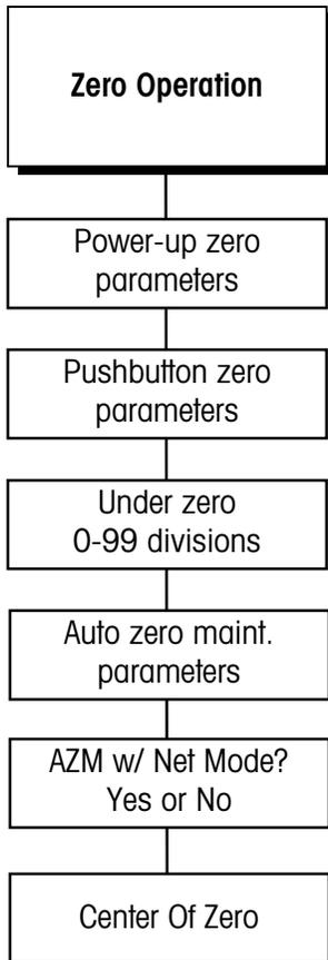
METTLER TOLEDO recommends that power-up zero be disabled by setting Positive and Negative range to 0% for scales such as tanks and hoppers which may lose power in the middle of a control process.
