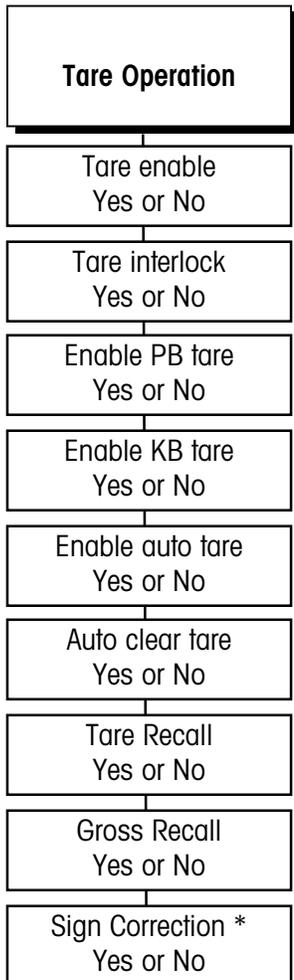
The Tare Operation sub-block lets you enable or disable the various tare options the LYNX terminal offers and in any combination. Three types of tare are available:
