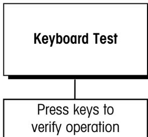
The keyboard test verifies the operation of each key on the LYNX terminal keypad.
