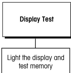
This sub-block tests the terminal's display and tests display ROM and RAM.
