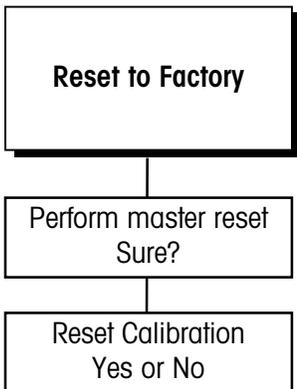
The Reset to Factory sub-block allows you to perform a master reset which returns all parameters for all program blocks to their original settings. To perform a master reset:
