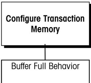
The LYNX terminal can store transaction data records in a transaction memory buffer to make them available for a host computer to acquire. The transaction memory buffer is 4,090 bytes long. This sub-block allows you to configure the LYNX terminal to behave in a prescribed manner should the buffer become full.
