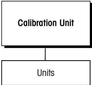
This sub-block lets you enter the units of measure to use when calibrating the scale and configuring capacity and increment size. Recalibration is required if you change the calibration unit.
