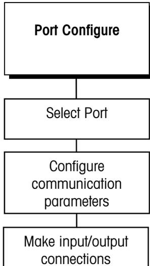
COM1 always has 1 stop bit. If COM1 is selected, the Stop Bits prompt does not appear.
