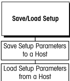
This sub-block allows saving from the LYNX terminal and loading to the LYNX terminal all setup parameters using a host device, such as a PC, connected to the LYNX terminal COM1 port. The LYNX terminal port COM1 must be configured to 2400 baud to correctly perform the "Load" function from the host (see the Serial Interface program block). The "Save" function baud rate is limited by that of the other device connected to COM1.
