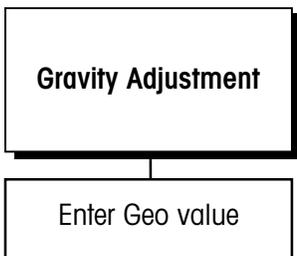
This sub-block is designed to let you enter a factor to compensate for gravitational differences between the factory calibration location and where the scale is currently located. If on-site calibration has already been performed, leave this value set to the factory default.
