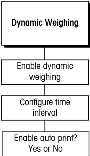
The update rate for an analog load cell system is 20 updates per second. The rate for DigiTOL scales is between 5 and 7 updates per second.
