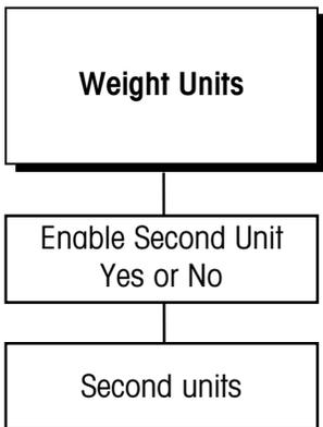
The Weight Units sub-block lets you select a second unit of measure for weight display, and enable or disable units switching. You can select a second weight unit from various pre-programmed standard weight units, or you can create a special weight unit with a custom name and conversion factor.
