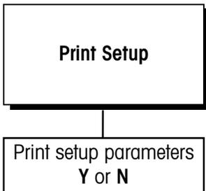
The Print Setup sub-block prints the terminal setup information as it is defined in the program blocks. It may be useful to have a hard copy of each terminal's setup parameters as back up. Print setup data will be sent out the port selected for demand output.
