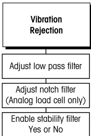
If the scale type is other than analog, the prompt for step 2 does not appear. Begin configuration with step 3.
