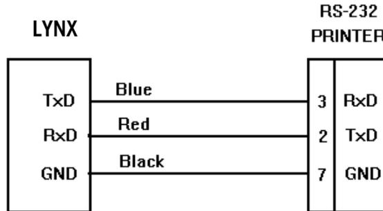
Figure 5-1 RS-232 Printer Cable Wiring
