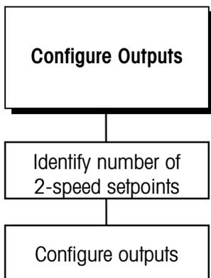
This sub-block lets you configure the LYNX terminal's five outputs for the required functionality. Outputs are found on the PAR2 discrete output connector. To simplify configuration, you must first select the number of 2-speed setpoints. Depending on the number of 2-speed setpoints, you then select the functions of the remaining outputs.
