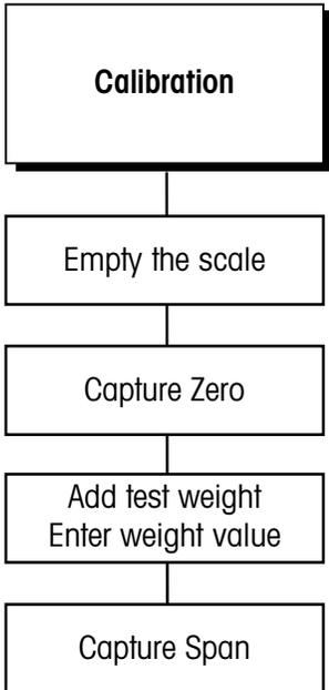
Calibration involves emptying the scale then placing a known test weight on an empty platform and allowing the LYNX terminal to capture values for zero and span. You can calibrate a scale with or without linearity correction. The LYNX terminal prompts you through the calibration.
