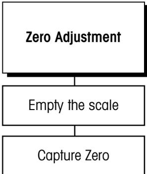
The zero value is the scale-empty reference as determined during calibration. The Zero Adjustment block lets you re-establish this value to compensate for any change since the last calibration. The scale must be empty before resetting the zero value.
