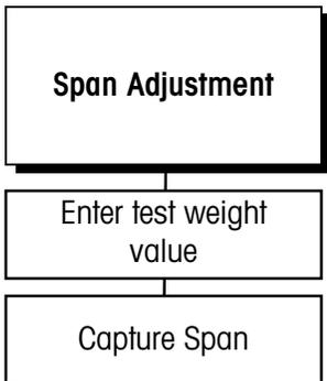
The Span Adjustment feature lets you make minor span adjustments without completely recalibrating the scale. Adjust the span by placing known test weights on the scale prior to entering span adjust. The terminal guides you through the procedure.
