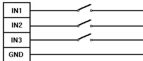
Figure 5-3 Standard Input Wiring
