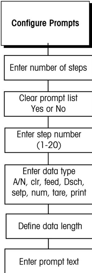
A prompt list displays a written sequence for an operator to perform a task while in Normal Operation mode. You can include up to 20 steps in a prompt list. The LYNX terminal has three preprogrammed prompts:
