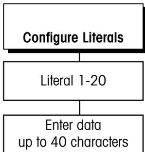
Literals are text strings such as site name or address that can be printed in a template. They can be up to 40 characters in length and are referenced by a field code. See the section entitled Configure Template Sub-block in this chapter. You can program up to 20 literals. To configure literals:
