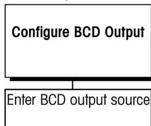
The BCD Output option kit provides up to six decades of TTL data. This sub-block lets you select the source data for BCD Output. To configure the sub-block:
