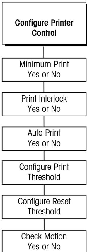
This sub-block lets you configure certain parameters that control when and how data is output to a printing device. These parameters apply generally to the LYNX terminal; they are not port specific. To configure the printer control sub-block:
