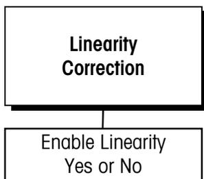
Linearity correction lets you calibrate the scale using calibration reference weights at mid-scale and full-scale ranges. Linearity correction allows for compensation of the non-linear performance of a load cell(s) or weighing system. If linearity correction is enabled, the calibration process requires additional steps. The terminal must be calibrated or recalibrated **after** you enable linearity correction.
