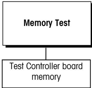
The Memory Test sub-block tests the terminal's internal memory. These diagnostics test the Flash memory, RAM, and EEPROM on the Controller board. The results of the memory tests are displayed on the terminal. To execute the memory tests:
