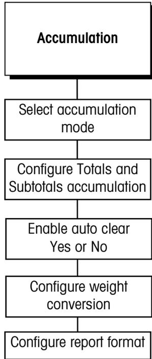
The LYNX terminal uses the primary weight unit (calibration unit) for accumulation.
