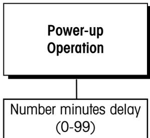
The Power-up sub-block lets you specify a time delay before the scale is operational. This delay allows a sufficient warm-up period for stabilization of the scale and load cell electronics. The LYNX terminal displays a count-down clock indicating the time remaining in the specified warm up period.
