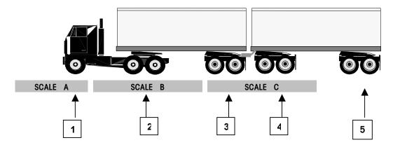
Position the truck so that the first axle is completely on a scale platform alone (no other axles are on that platform also). In the example above, Axle 1 is on scale A with no other axles.
