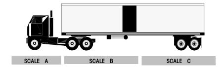
The truck leaves the scale and then returns after loading or unloading its cargo.
