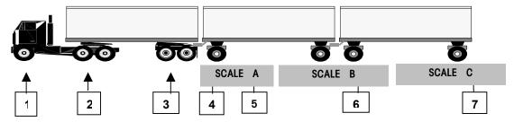
In the example, Axle 5 is now positioned on Scale A by itself.
