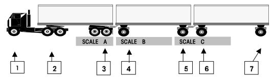
Axle 3 is now positioned on Scale A by itself.
