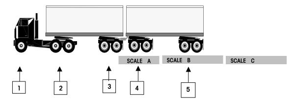
Axle 4 is now positioned on Scale A without any other axles.
