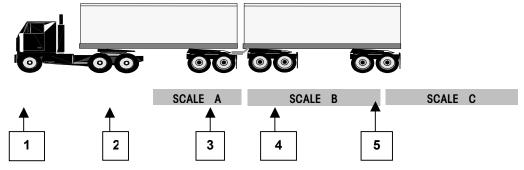
Axle 3 is now positioned on Scale A without any other axles.
