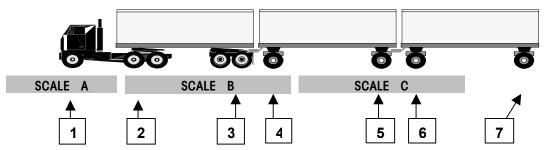
Position the truck so that the first axle is completely on a scale platform alone (no other axles are on that platform also). In the example above, Axle 1 is on scale A with no other axles. Once Triple Mode is selected, follow the directions.
