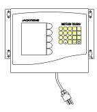
The JXHG (harsh environment terminal version) is comprised of a JAGXTREME chassis and a graphical display housed in an enclosure. For additional information, refer to the section on the blind JAGXTREME terminal in the JAGXTREME Terminal Technical Manual.
