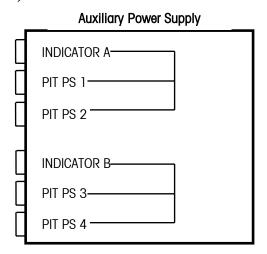
The purpose of the auxiliary power supply is to provide two identical circuits, each with a 24 VDC power supply output capable of driving up to two pit power supplies. Each pit power supply can drive a maximum of 12 load cells. As shown above, the INDICATOR A and B inputs are connected to the pit PS outputs. The two circuits are completely isolated. The only exception is the same 24 VDC power supply output being used for pit PS1 and 3. The second 24 VDC supply is shared between pit PS2 and 4.
