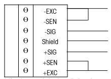
$<sup>^{*}</sup>$  If an increase in load results in a decrease in weight display, reverse the signal wires (+SIG and -SIG).
