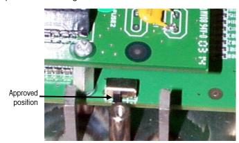
Figure 2-2: Metrology Switch in the Approved Position
