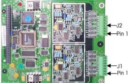
Figure A-6: Single (left) and A/D (right) Board Connector Locations
