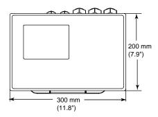
Figure 1-2: Top View of IND310drive
