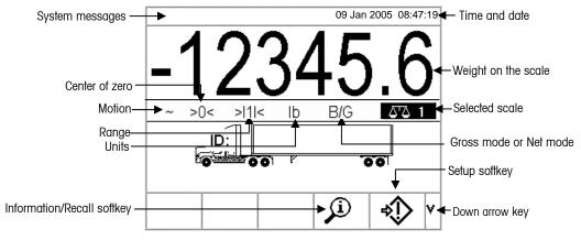
Figure 2-6: Default Vehicle ID Weighing Operation Screen
