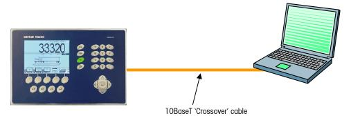
Figure B-1: Connecting the IND310drive to a PC with a Crossover Cable
