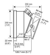
Figure 1-3: Side View of IND310drive
