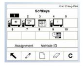
Add or rearrange the softkeys on the terminal's main menu on the softkeys setup screen. When the softkeys setup screen opens, focus is on the softkey position numbers located above the icons.
