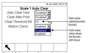
Figure 3-5: Setup Screen (Focus on Field Value)
