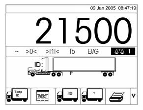
**Figure F-2**: Example of the First Softkey Screen (Total of Ten Softkeys Available)
