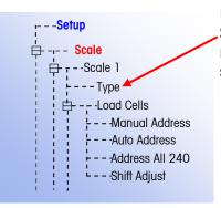
Legal for Trade settings are accessed through the setup menu in Scale/Scale1/Type. The IND310drive operates within the weights and measurement rules associated with the Legal for Trade settings. To change the Legal for Trade settings:
