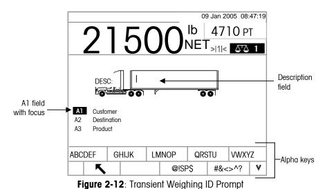
3. Use the alpha keys and the numeric keypad to enter the description. Press the ENTER key to complete the entry. To continue the transaction, see Outbound Process.
