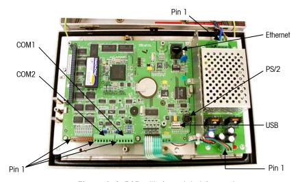
Figure A-4: PCB with Associated Connectors
