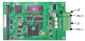
Figure A-9: POWERCELL Board Connector Locations
