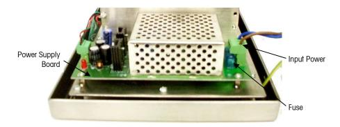
Figure A-5: Power Supply Board
