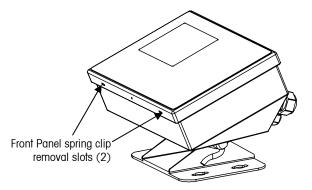
Figure A- 2: IND310drive Terminal Access
