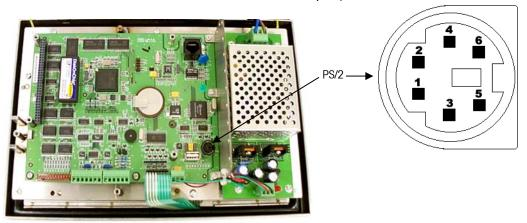
Figure 4-2: PS/2 Connector on the Main PCB and Pin Locations
