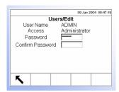
Press the EDIT softkey to access a second screen where a password can be entered.
