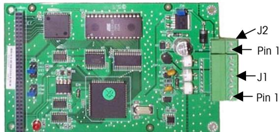
**Figure A-9:** POWERCELL Board Connector Locations
