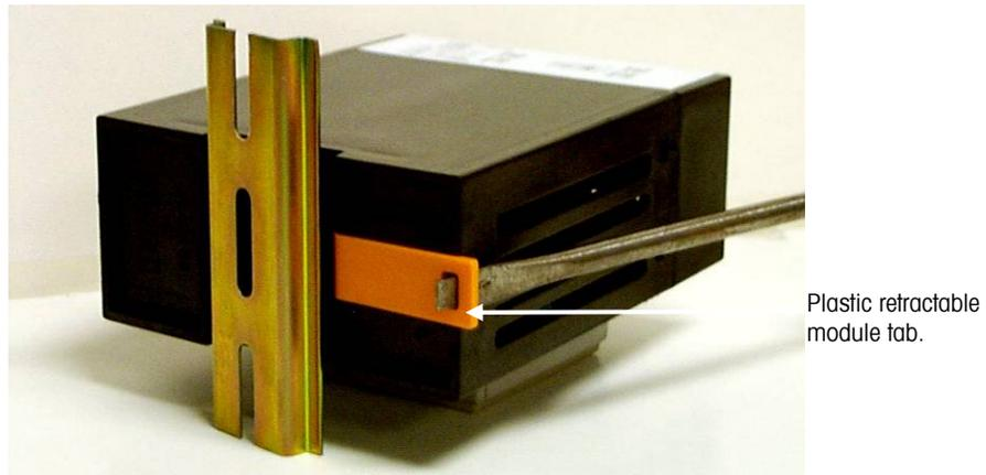
**Figure A-4: Plastic Retractable Mounting Tab**
