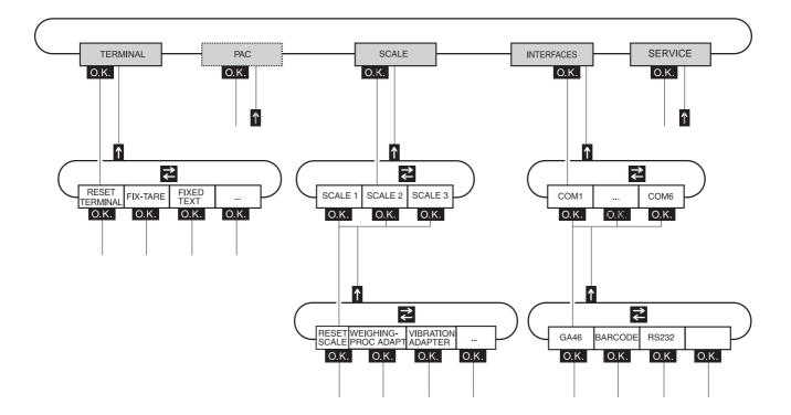
**TERMINAL** For system settings, such as entering the date and time or loading permanent texts, see section 4.3.2.
