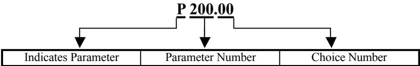
For example, parameter 200 is a selection parameter that holds the baud rate for the serial. This is a selection parameter because a choice number between 00 and 06 must be used. Each choice number corresponds to a different baud rate. To change the baud rate from the default value of 9600 to 4800, perform the following steps from the Setup Mode.
