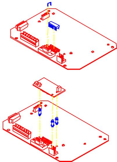
Figure 6-8: RS-485 Installation
