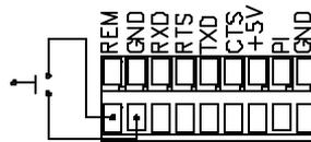
*Figure 2-9: Remote Key Connection (Model 350 stainless and Model 355)*
