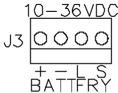
*Figure 6-14: Model 350/355 Main Board Battery Connection*
