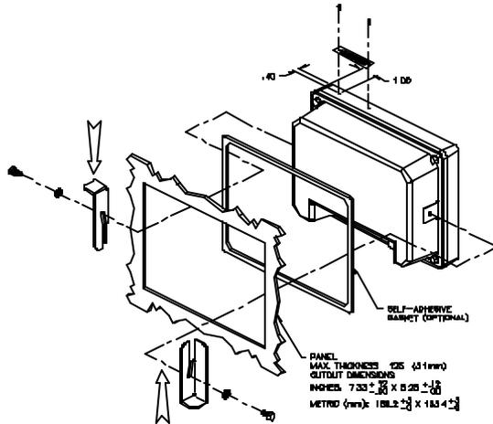
*Figure 6-2: Model 350 Panel Mount Installation (Die Cast Model)*
