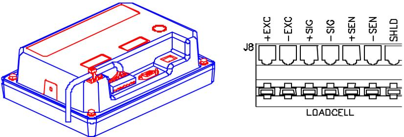
*Figure 2-6: Cable Tie on Die Cast & Connector (J8)
