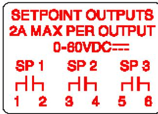
*Place this label above the setpoint card knockout (die cast)*
