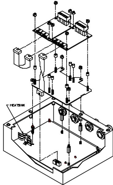
*Figure 6-6: Option Board Installation
