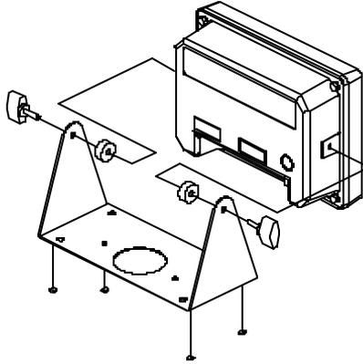
*Figure 6-1 Swivel Bracket Installation (Die Cast Model)*
