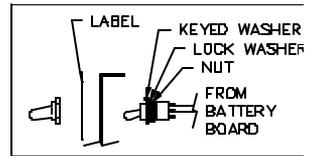
Figure 6-12: Battery Option Installation (Stainless Steel Enclosure)
