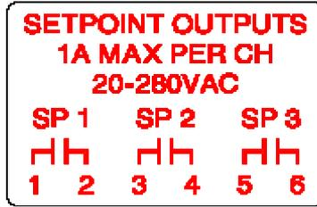
Place this label above the setpoint card knockout (die cast).
