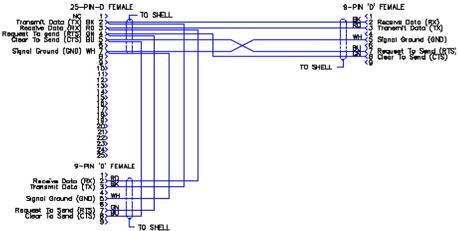
Figure 2-7: GSE Serial Cable, Part Number 22-30-29752
