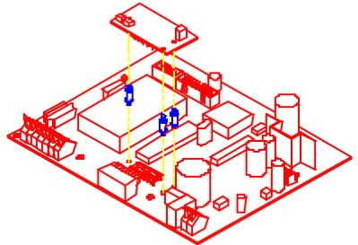
*Figure 6-9: RS-485 Installation
