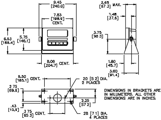
Figure 2-2: Model 350 Zinc Die Cast Front Dimensions
