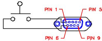
*Figure 2-8: Remote Key Connection (Model 350 die cast)*
