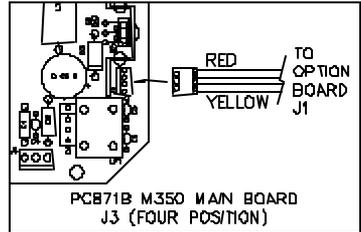
Figure 6-13: Battery Option Installation (Die Cast Enclosure)
