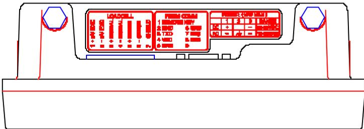
Figure 2-5: Model 350 Zinc Die Cast Enclosure Wiring Label
