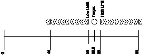
Figure 3-2: Example #1 Bargraph Segments (Weighted Value)
