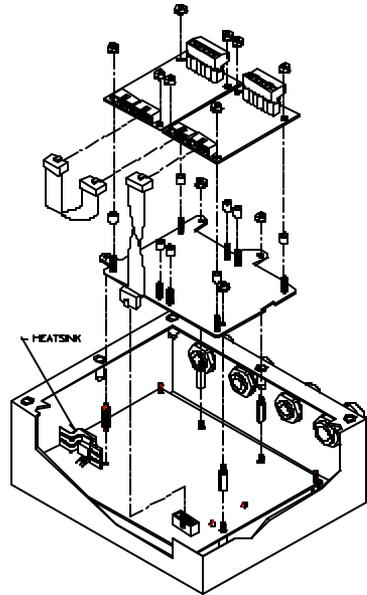
*Figure 6-4: Option Board Installation
