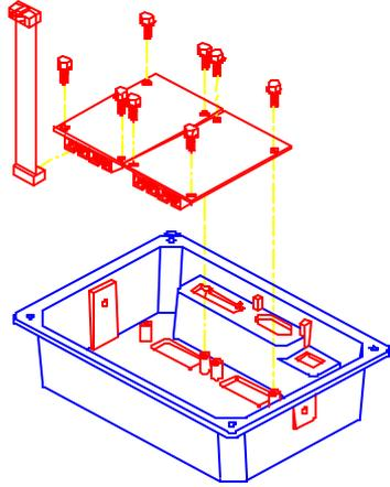
*Figure 6-5: Option Board Installation
