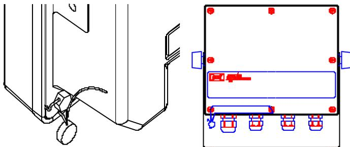
Figure 5-3: Physical Seals (Zinc Die-Cast / Stainless Steel)
