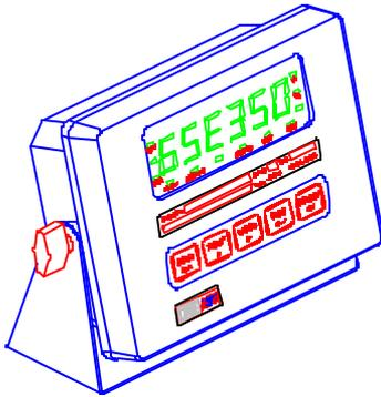
The optional mounting bracket allows the zinc die cast enclosure to be securely fastened to another surface. The bracket is attached to the indicator with two thumbscrews and can be swiveled to an optimal viewing angle.
