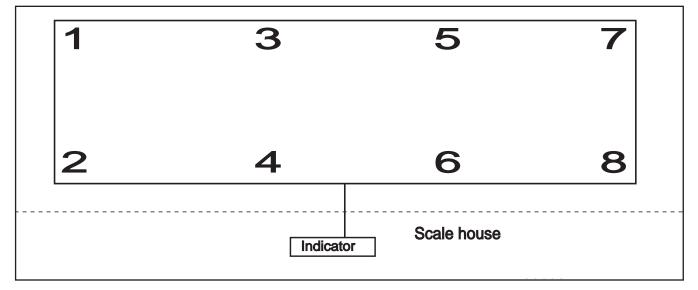
**Note:** Intalogix<sup>™</sup> installations utilize a specific numbering system for load cells because of digital addressing of the SSCs.
