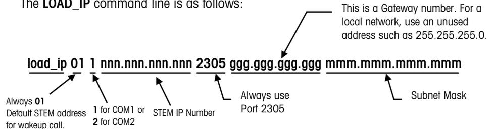
The gateway number may be required to access a host PC on another network. Check with your IS department for details on a gateway and submask number.
