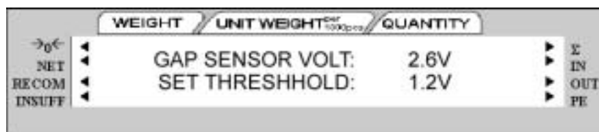
Figure 3-7. Gap Sensor Voltage Adjustment
