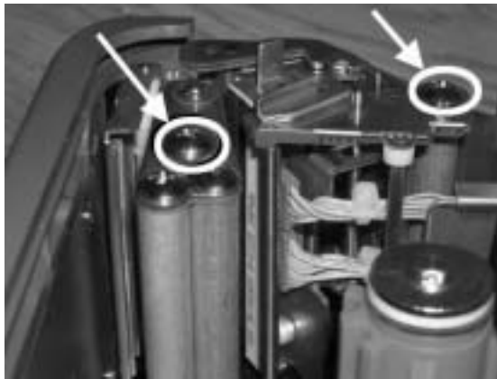
Figure 4-16. Printer Head Assembly Screw
