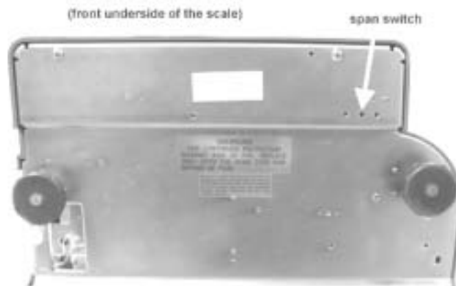
Figure 2-4. Location of Span Switch
