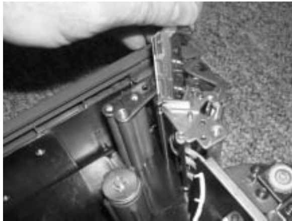
Figure 4-19. Removing the Thermal Print Head
