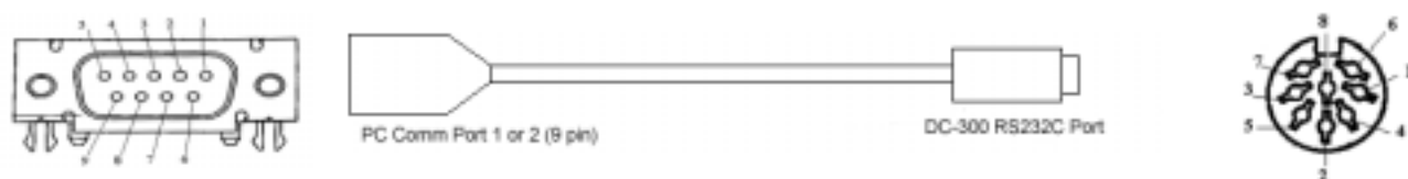
Figure 6-15. Connection from Scale to PC
