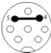
Figure 3-1. Test Connector for RS-232 Ports
