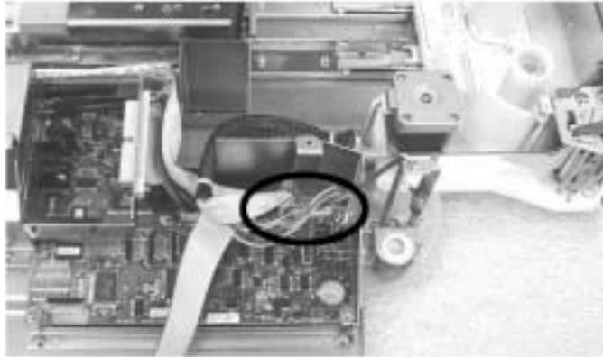
Figure 4-13. Disconnect Printer From Main Board
