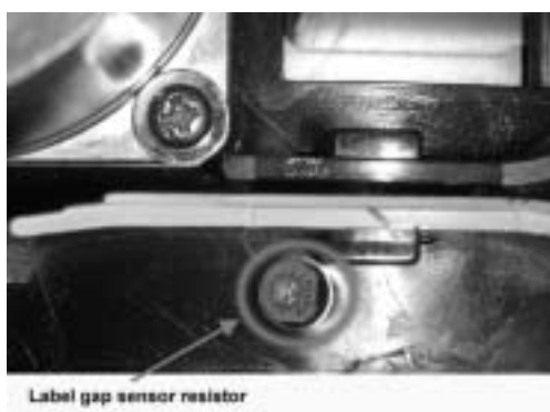
Figure 3-6. Label Gap Sensor Resistor Location
