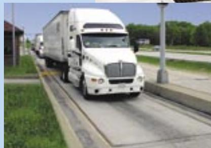
*Modules may be marked with a painted edge stripe to assist the driver in properly positioning the truck. Each section functions as an independent scale.*
