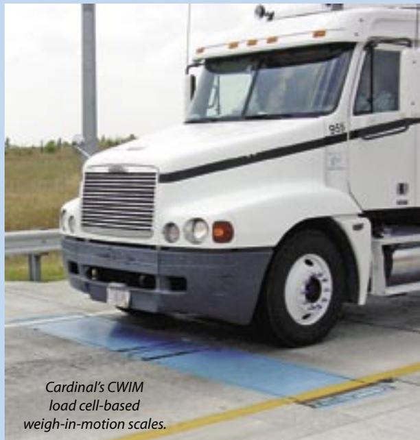
*Cardinal's CWIM load cell-based weigh-in-motion scales.*
