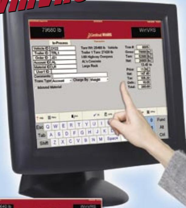
*WinVRS Featuring the Ease of a Plasma Touchscreen Display Without the Need for a Separate Keyboard.*
