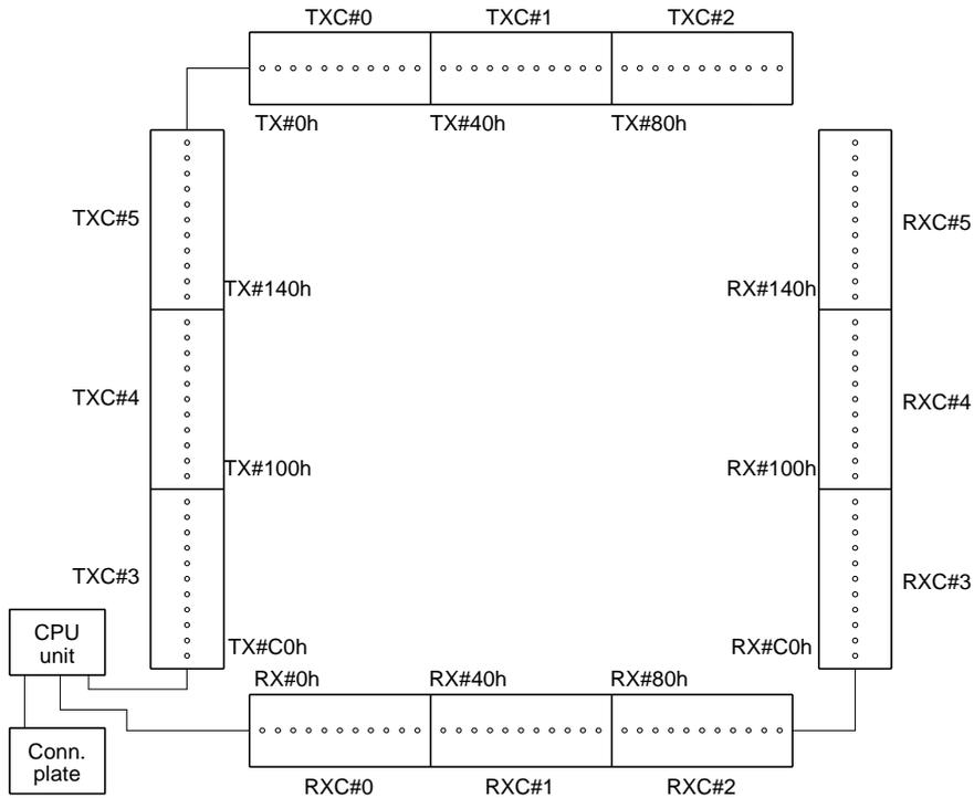
The figure shows how boards and pixels are numbered on a 96\*96 cm Frame. On the figure we have:
