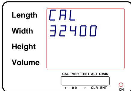
The tacho rate, here 32400 pulses/meter is displayed.
