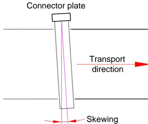
The skewing angle has its corner point on the connector plate side of the Frame, and it is defined as positive when the Frame is "pointing" in the same direction as the transport direction, as described in the figure above.
