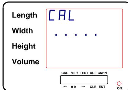
Start the conveyors and let the calibration object go through the Frame. The calibration object must be oriented along the transport direction as shown below:
