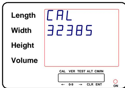
New calibration rate in pulses/meter is displayed.
