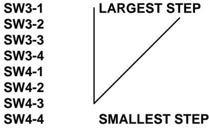
Turning ON any of the SW3 and SW4 Span switches will decrease the weight indication. SW3-1 has the greatest effect. SW3-3 has 1/2 the effect of SW3-1. SW3-3 has 1/2 the effect of SW3-2 and so on through SW4-4.
