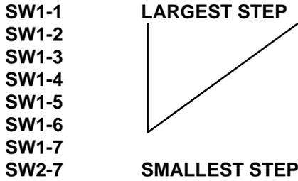
Turning ON any of SW2 Span switches will decrease the weight indication. SW1-1 has the largest effect. SW1-2 has 1/2 the effect of SW1-1. SW1-3 has 1/3 the effect of SW1-2 and so on through SW2-7.
