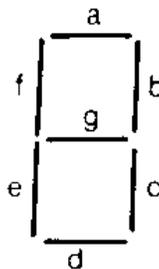
To confirm that this checking system is functional, the Test Verify pushbutton, if equipped, causes a short in one of the LED segments which results in false data, and a display verify failure indication.
