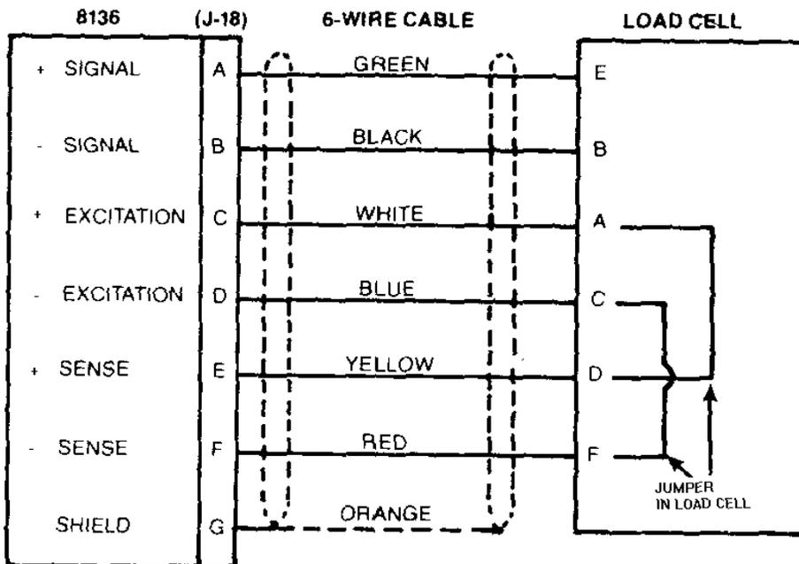
SINGLE 6 WIRE CELL CONNECTED DIRECTLY TO INSTRUMENT.
