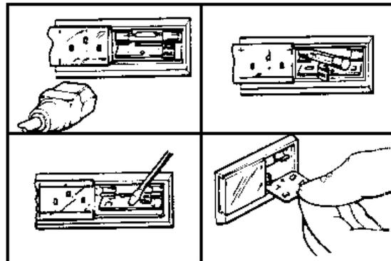
3. With the fuse removed, use a small screwdriver or similar object and gently pry the card from the assembly. A hole in the card is provided to assist removal.
