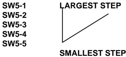
Turning On any of SW5 initial switches will increase the initial compensation. SW5-1 has the largest effect. SW5-3 has 1/2 the effect of SW5-2 and so on down to SW5-5.
