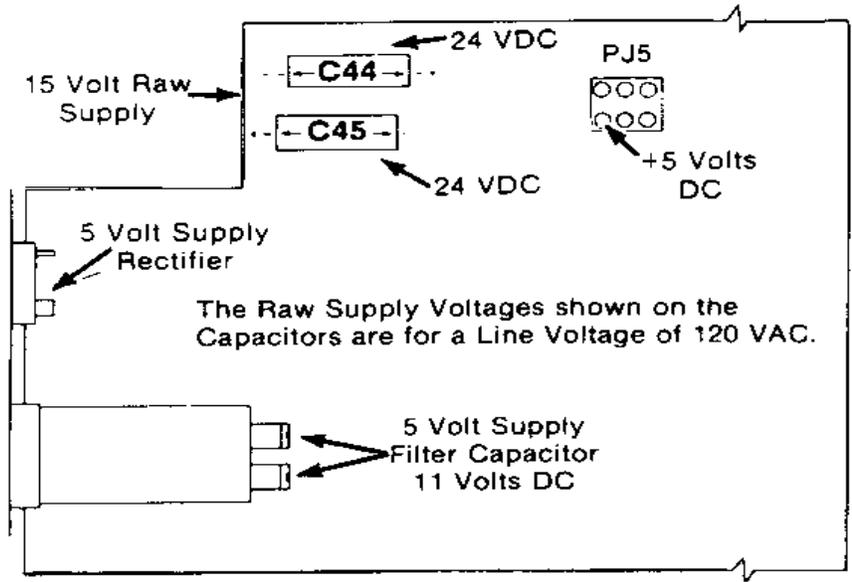
**NOTE: On the 11411100A PCB, C44 and C45 will be labeled C52 and C51 respectively.**
