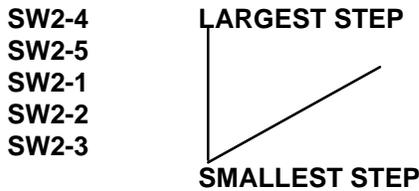
Turning ON any of the initial switches will increase the initial compensation. SW2-4 has the greatest effect. SW 2-5 has 1/2 the effect of SW2-4. SW2-6 has 1/2 the effect of SW2-5 and so on down through SW2-3.
