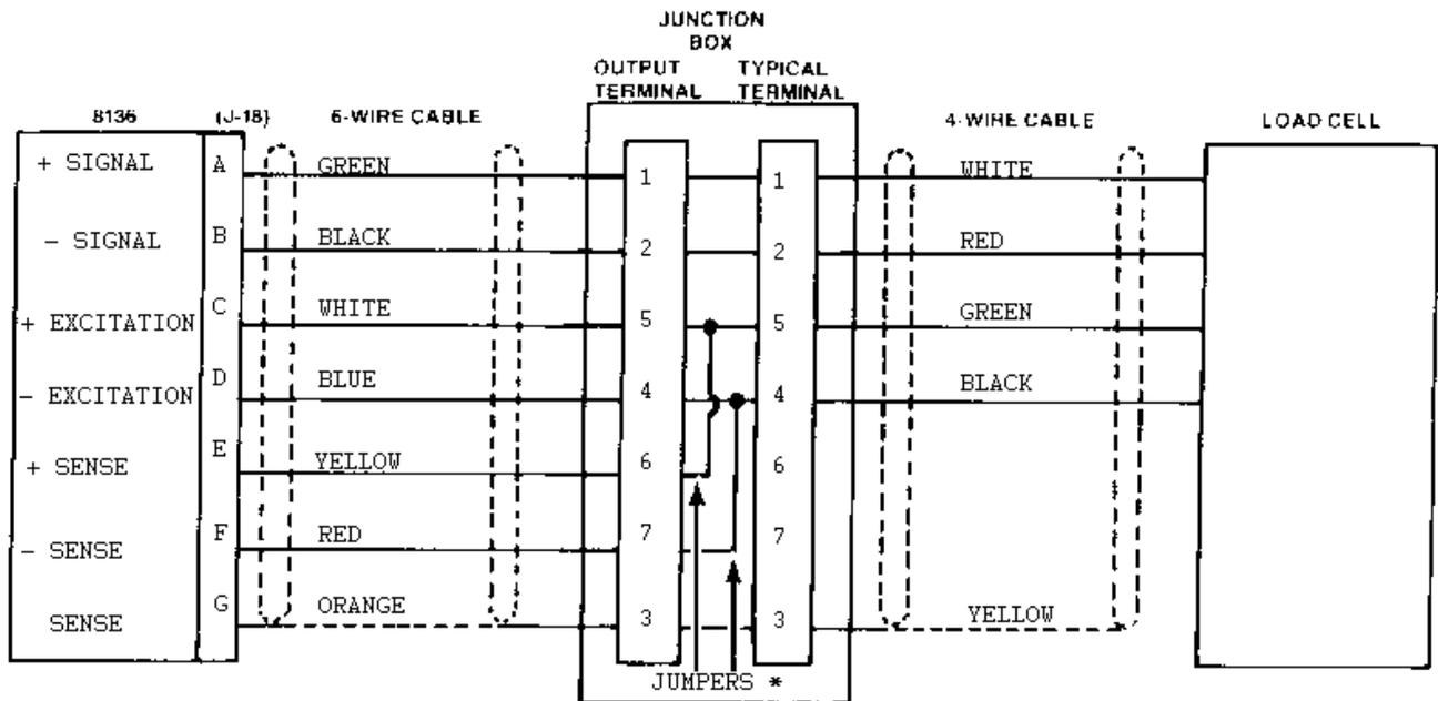
\* When using 4 wire cells, there will be jumpers between terminals 4 and 7 and between terminals 5 and 6 on TB101. On the 6 wire cells the jumpers are built into the load cell and they are between pins A and D and between pins C and F. Use terminal strip TB101 if only one load cell is used.
