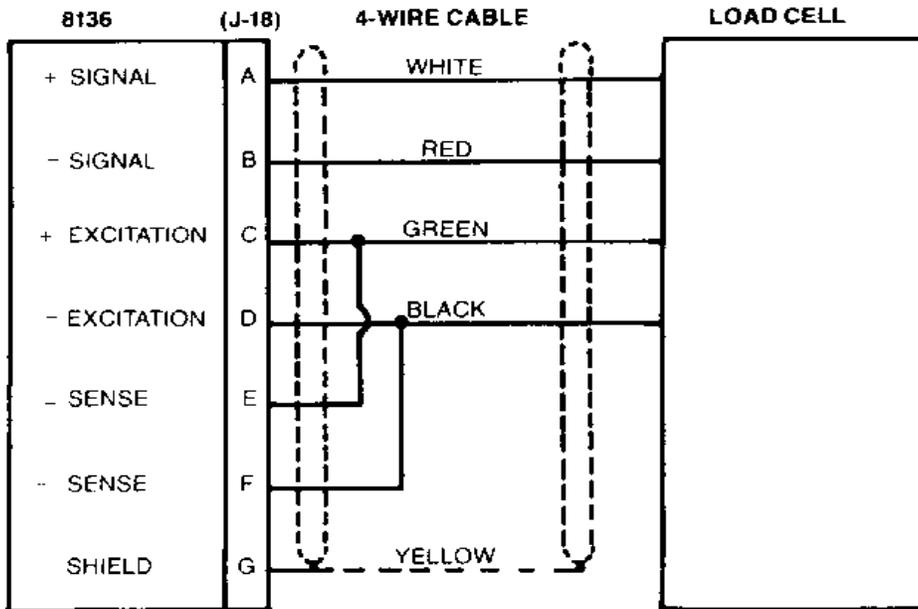
SINGLE 4 WIRE CELL CONNECTED DIRECTLY TO INSTRUMENT.
