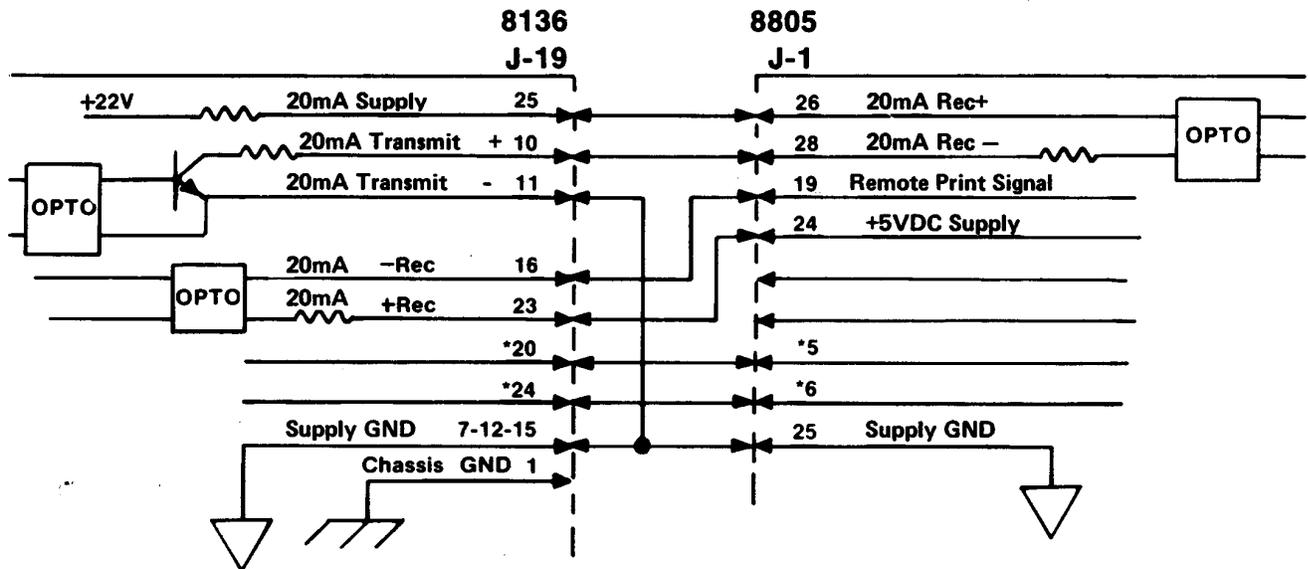
\* Wire is connected in cable but used for 8132 only.
