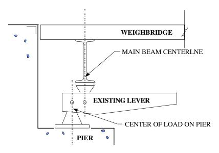
Figure 2-a: Typical Lever Corner Assembly
