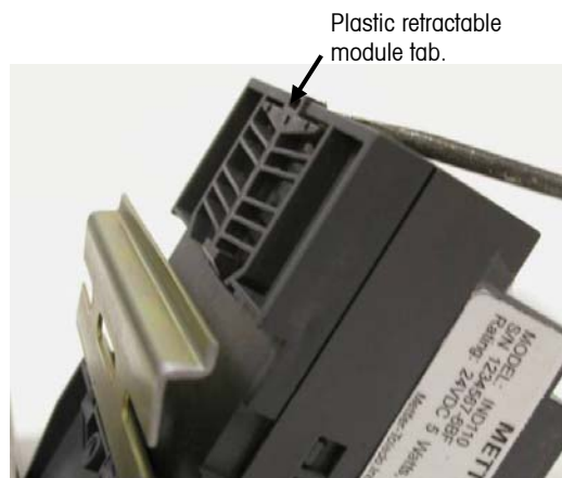
Figure 2-2: Retracting the Module Tab
