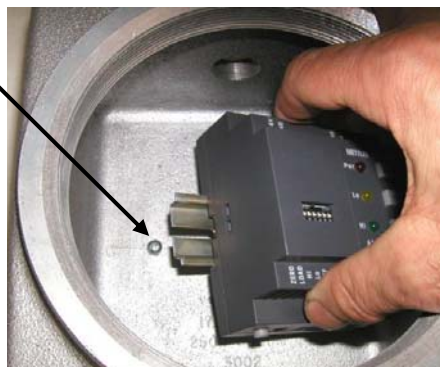
Figure 3-3: Sliding the DIN Rail Slot Onto One Screw
