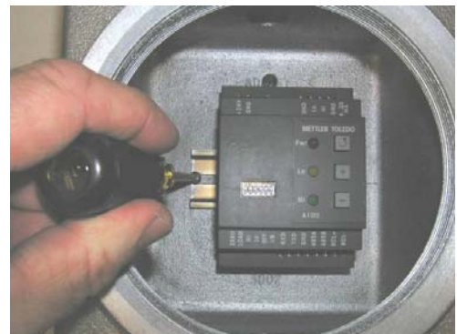
Figure 3-4: Securing the DIN Rail
